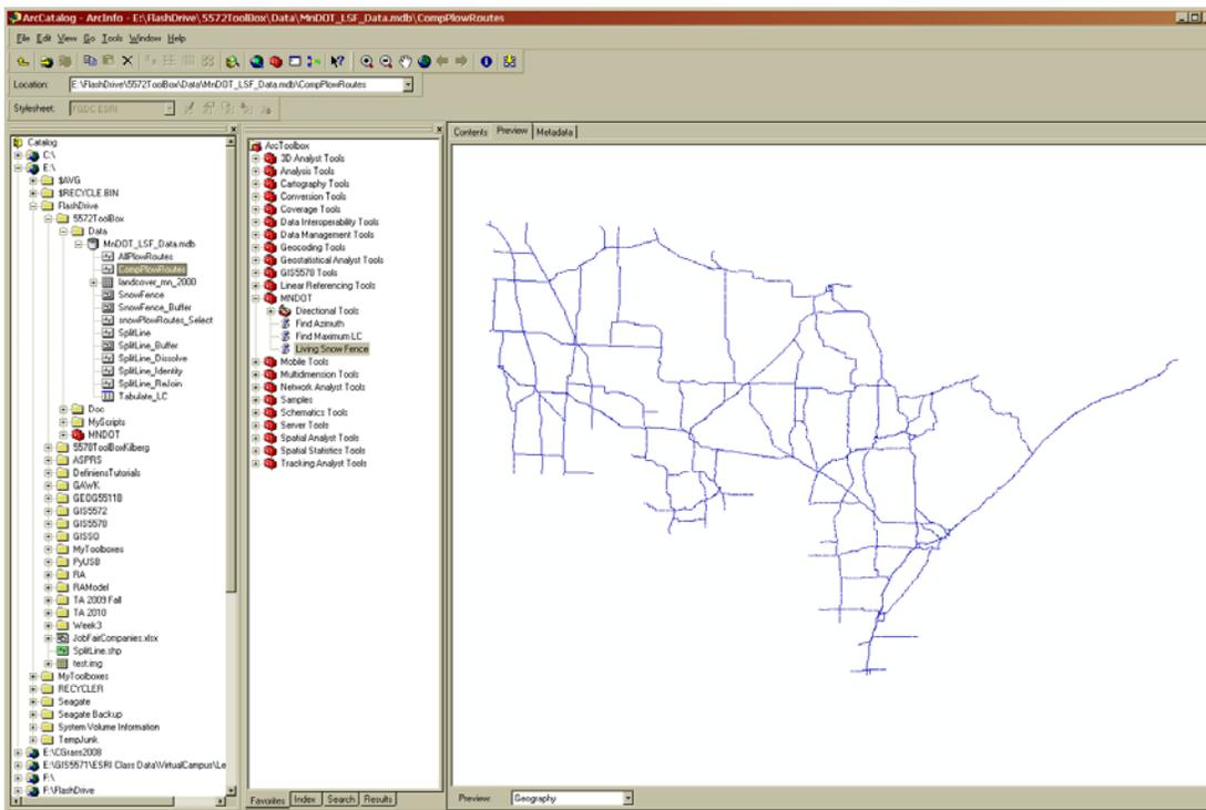
The following screen shows an example of the data that is added to the base Plow Route file at the end when a snow fence is found impacting this section of roadway. The azimuth field shows that azimuth between 0-179°. The MaxLC field gives the predominant land cover class that
