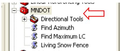
Note: the Find Azimuth and Find Maximum LC tools are used by the Living Snow Fence tool. You will not execute them directly.
