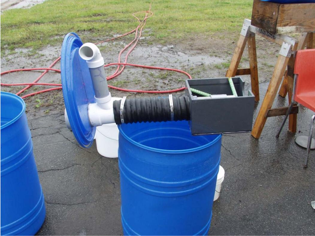
**Figure 5.3: Transverse Drain and Flow-Out Meters**
