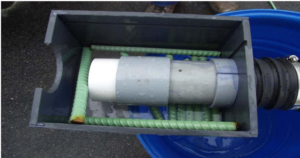
**Figure 5.4: Flow-Out Meter Partial Assembly**
