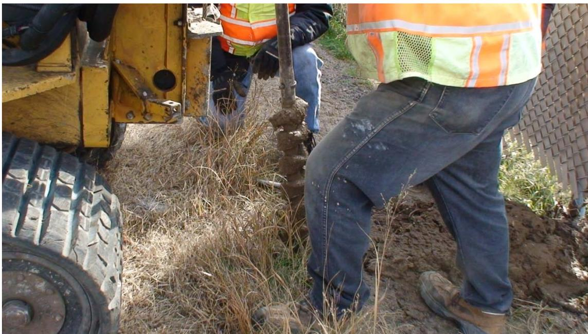
**Figure 2.16: In the Water Bearing/Saturated Layers, Auger Sample-Retention Was Minimal**
