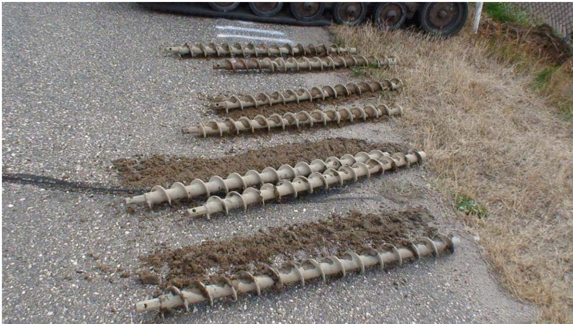
**Figure 2.13: Well 2 Encountered Saturated Sands Up to 30 Ft Depth below Surface**
