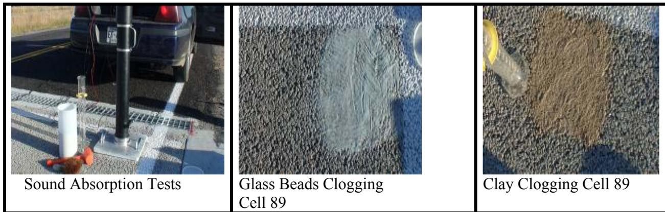
**Figure 9.8: Accelerated Clogging Test**
