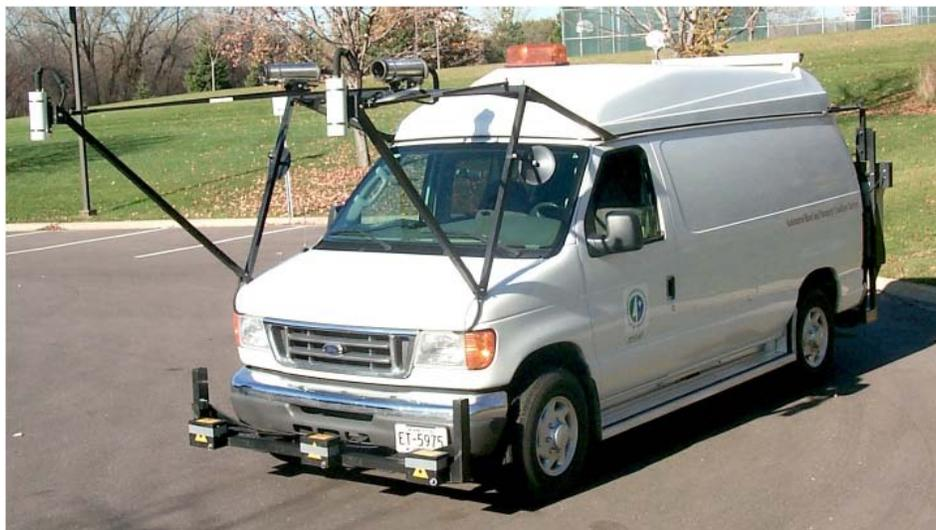
**Figure 6.2: Digital Inspection Vehicle**
