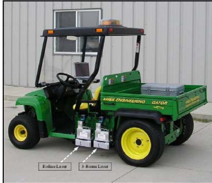
**Figure 6.1: Lightweight Inertial Surface Analyzer**
