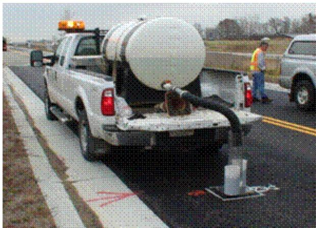
**MnDOT Infiltrometer Test**
