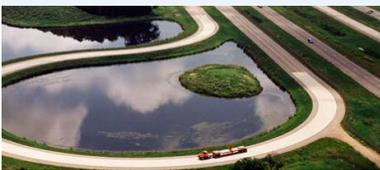
The MnROAD facility consists of two roadways instrumented with thousands of sensors that record traffic load response and environmental data.
