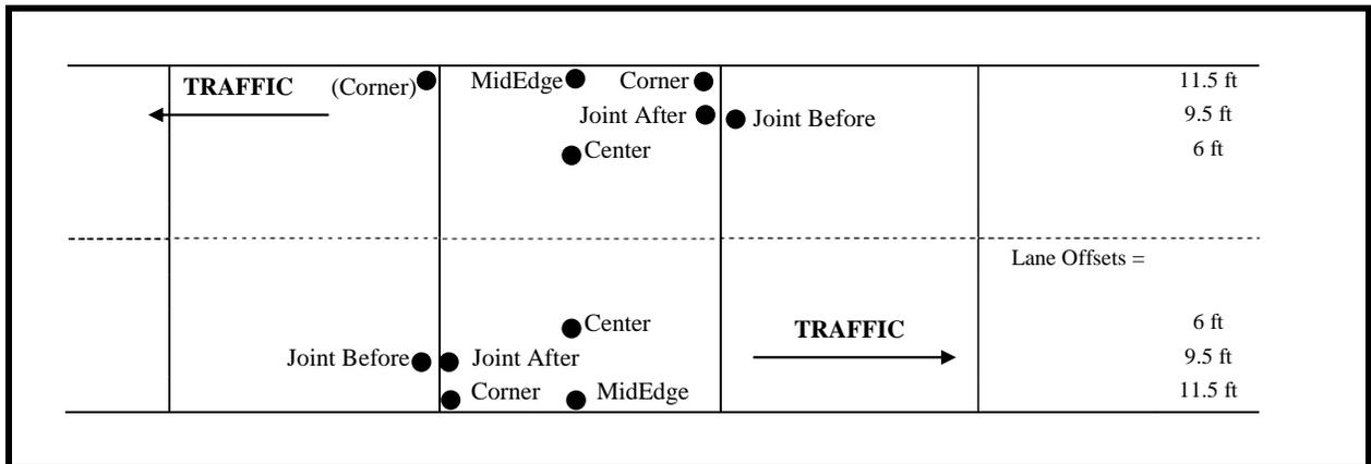
Figure 15. Diagram of FWD test points in a typical LVR cell.
