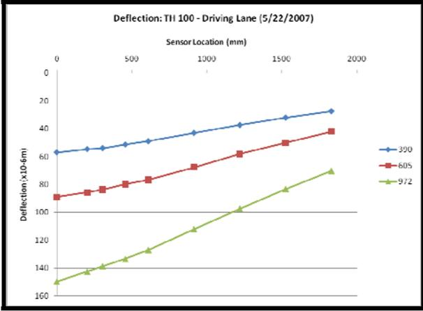
Figure 17. Deflection of a TH 100 Pavement of similar thickness design.
