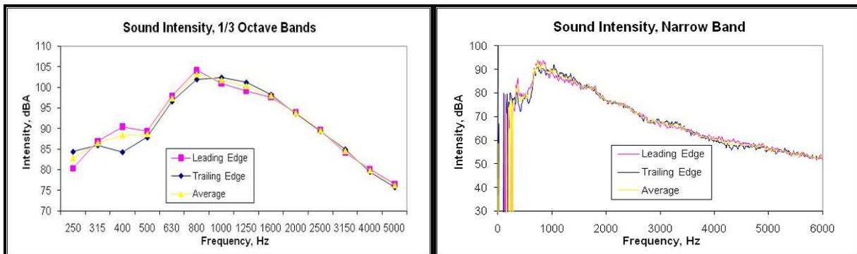
Figure 6. Typical sound intensity graphs from OBSI data, Cell 39.
