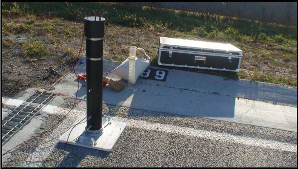
Figure 7. Mn/DOT BSWA 435 sound absorption testing device, Cell 89 (ASTM E-1050).
