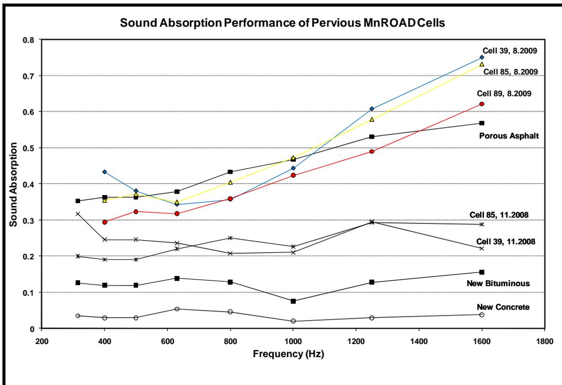
Figure 8. Absorption value plot for various MnROAD cells.
