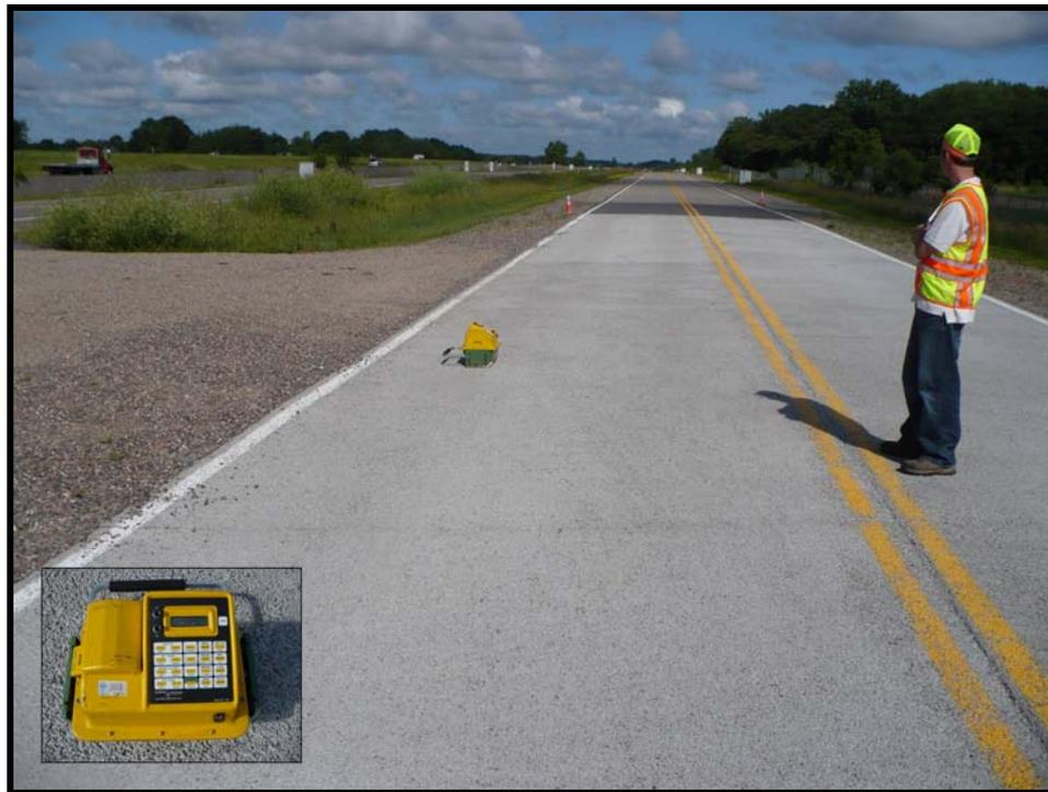
Figure 2. Nuclear backscatter density testing on Cell 39.
