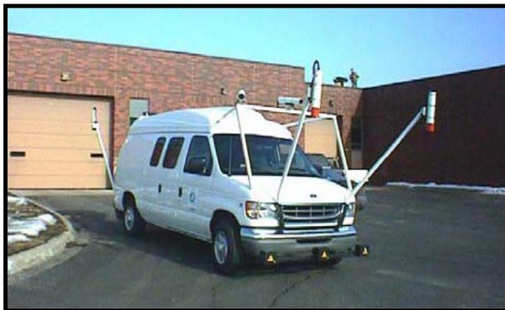
Figure 13. Pathways High Speed Laser Equipped Surface Evaluation Device (ASTM E-950).
