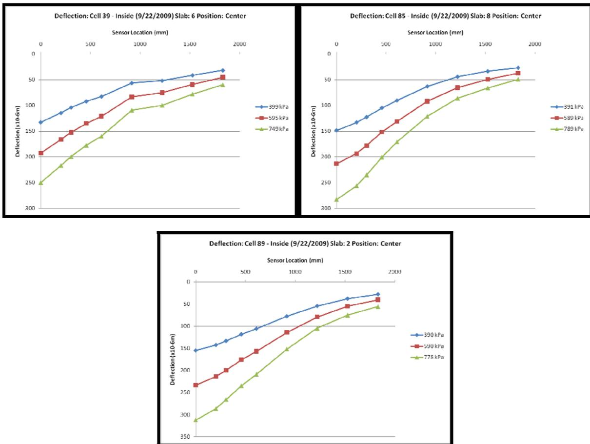
Figure 16. Representative deflection basins for Pervious Concrete Cells.
