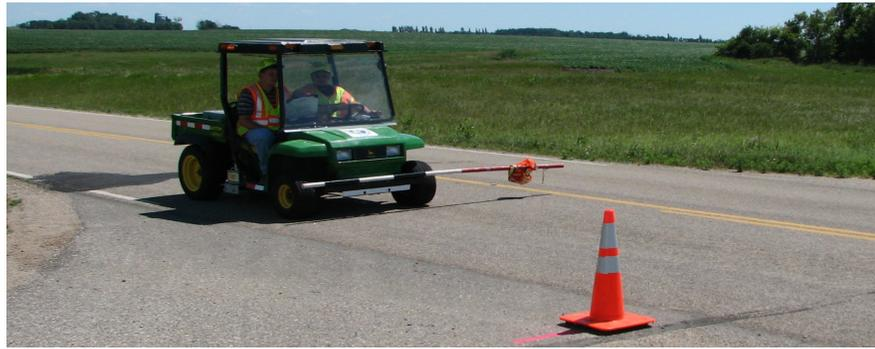
IRI algorithms for calculating ride quality from pavement profiles use data from inertial profilers, which use laser sensors to take precise measurements per inch of pavement.
