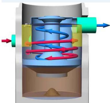
Water enters a hydrodynamic separator, swirls and then exits with captured sediment settling at the bottom of the chamber.
