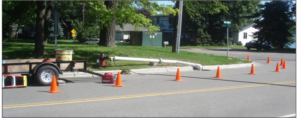
For the field test, water was piped from a fire hydrant directly into a storm sewer catch basin with a valve to adjust the flow rate. From the catch basin, the water flowed through a storm sewer pipe under Rice Creek Road to another catch basin, and then into the V2B1 hydrodynamic separator. Water flow and washout sediment exiting the device were measured.
