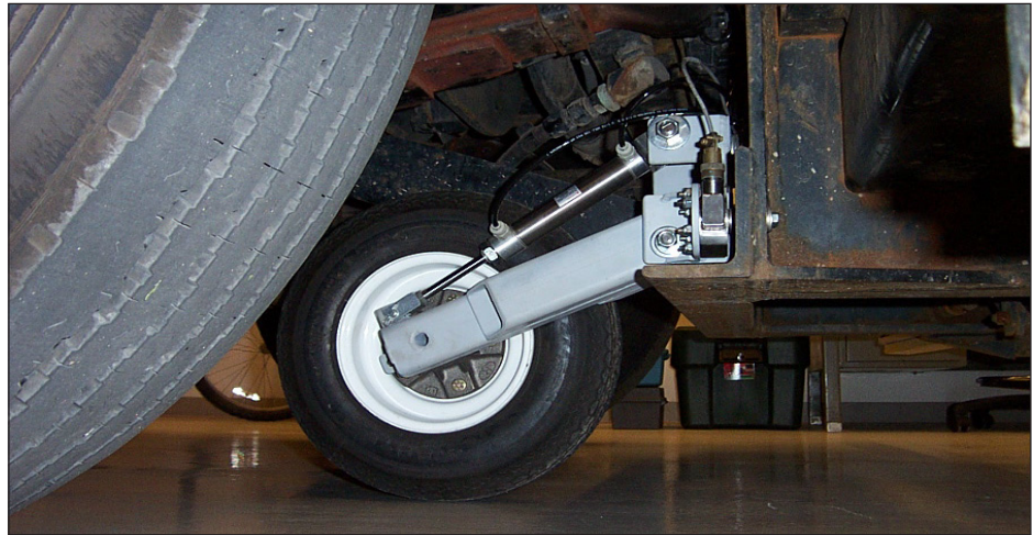
A small, redundant wheel located near the front axle of the snowplow uses sensors and unique technology to measure friction under a wide range of operating conditions.
