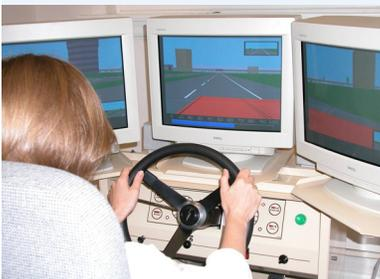
The driving simulator console had three 17-inch CRTs, a steering wheel and pedals, and an automobile seat. Speakers behind the CRTs simulated engine noise.
