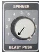
11 Turn spreader knob down to zero for safety
