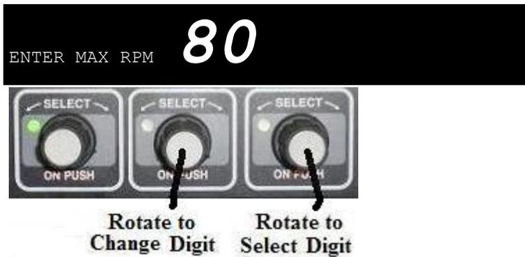
Note: Example RPM values are about 80 RPM for a 6" auger and about 180 RPM for a 9" auger (these may vary)
