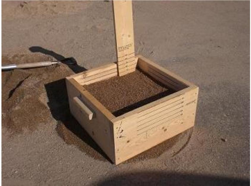
**Bottomless Box - No Lifting** - Box is bottomless, so no lifting is required. Easy to pull box off. Optionally add marks at i.e. 80% full, 90% full, etc.
