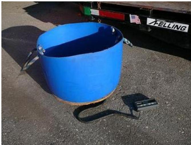
**Weight Box** - Large box that automatically weighs material. Can collect approximately 500 pounds. **Requires a skid steer or fork lift** for positioning and emptying. Simple to use.
