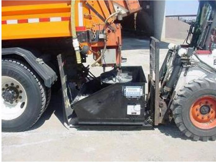
**Weight Box Meter** - Zero meter before dumping. Read weight after dumping.
