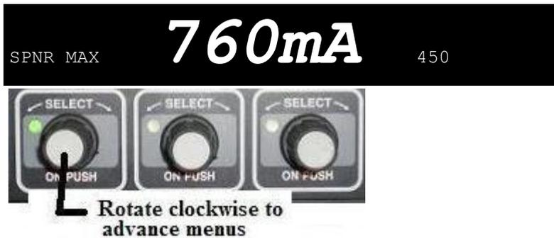
7 Spinner RPM (**450** in picture) will be displayed on screen
