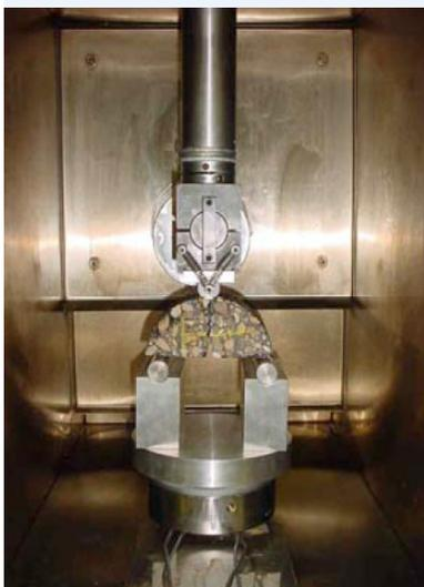
In the Semi-Circular Bend test, a load is applied to a halved asphalt mixture core sample while gages are used to record resulting cracks.
