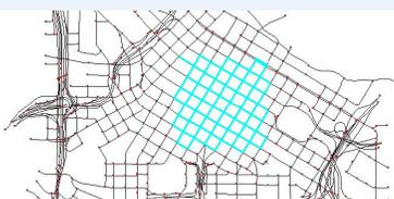
This screen shot from the evacuation software tool shows how the extent of the user-specified disaster area is highlighted after the user enters the desired radius.
