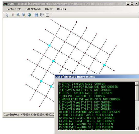
In this screen shot from the evacuation software tool, the signaled intersections selected for officer deployment are highlighted on the map. A list of all network signaled intersections identified as “CHOSEN” and “NOT CHOSEN” appears in the “List of Selected Intersections” window.
