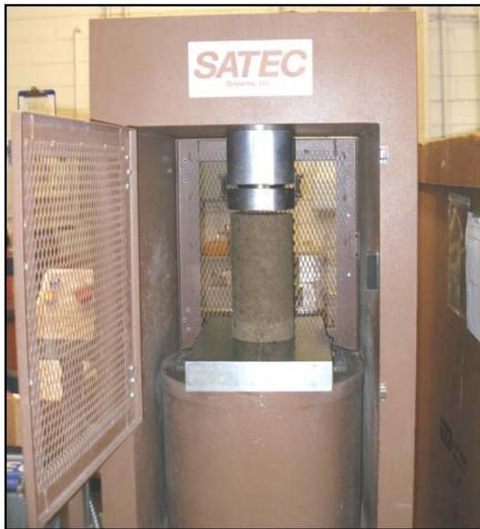
**Fig. D.4. Unconfined compression testing equipment.**
