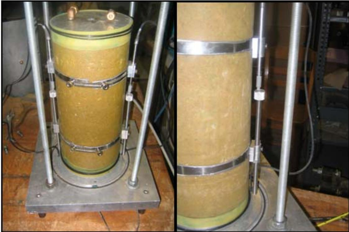
**Fig. 4. Internal LVDT clamps mounted on a resilient modulus specimen.**
