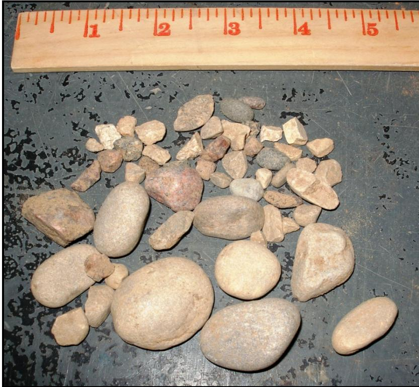
**Fig. 7. Photograph of gravel content from a sample of Class 5 base.**
