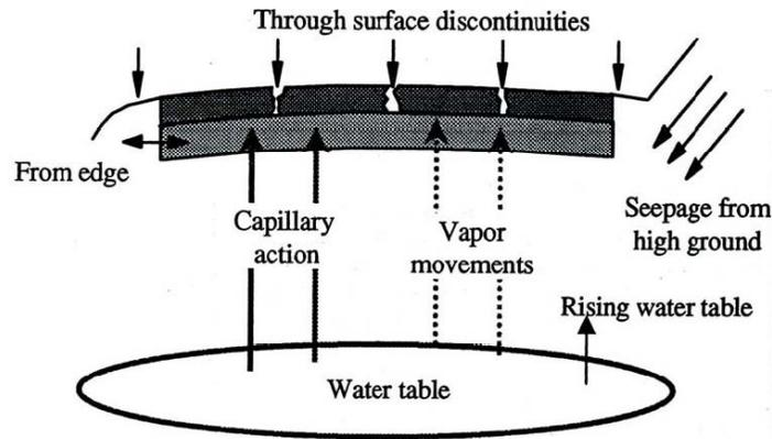
This diagram depicts avenues for moisture to reach the subsurface of a roadway. The main source of water infiltrating into pavement structural sections is from precipitation.
