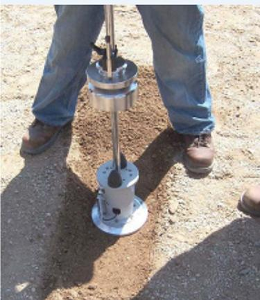
LWDs determine stiffness by measuring the deflection of the ground induced by a dropped weight.
