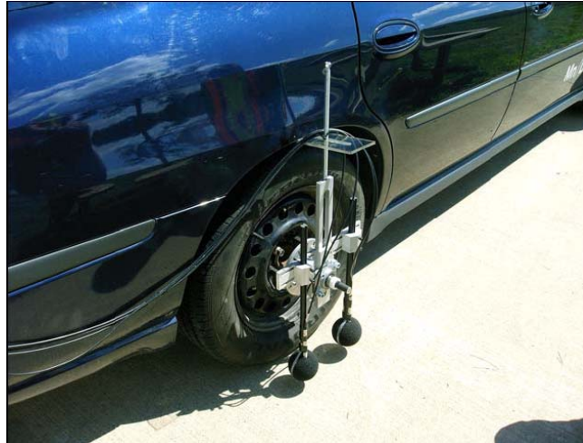
Figure 1. Mn/DOT OBSI Set-Up. Rig System by Illingworth & Rodkin, Microphones from BRC/ GRAS and Front End Analyzer from Bruel & Kjaer. (OBSI was invented by Dr. Paul Donovan of Illingworth & Rodkin. The system is mounted on a Model 2006 Chevrolet Impala using a Standard Reference Test Tire in the rear right wheel.
