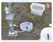
Researchers measured the water infiltration rate and soil strength to assess the effectiveness of the tilling procedures.
