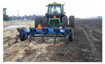
Investigators used three plows—with varying tine depths and tine types—to till the soil types examined in the project. The DMI chisel plow (shown above) operates at 12 inches deep.
