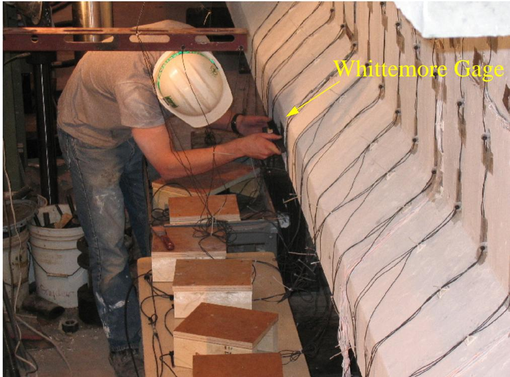
**Figure 4.20 Measurement of DEMEC Points**
