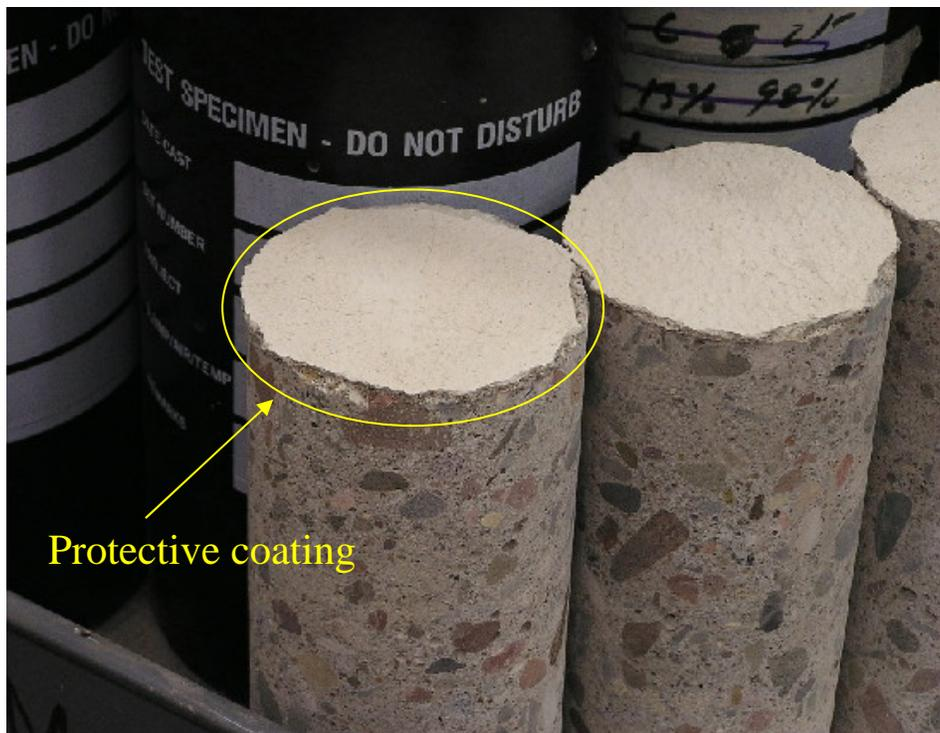
**Figure C.2 Protective Coating on Cores**
