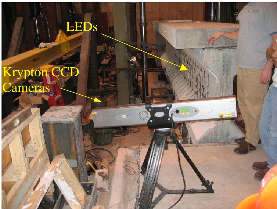
**Figure 4.17 Krypton Setup up for Specimen I**
