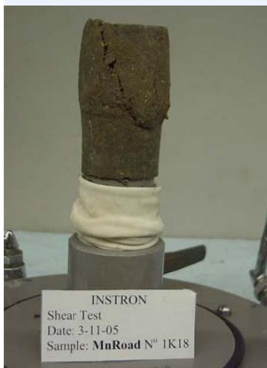
Researchers tested soils in the laboratory to correlate suction (how tightly water is held between soil particles) with properties like shear strength.
