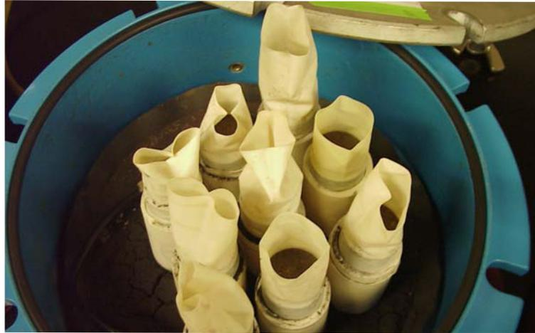
To bring soil specimens to a given level of soil suction, the specimens were placed in rubber sleeves and put in a pressure chamber.
