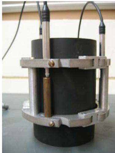
Figure 3.7: Synthetic Specimen
