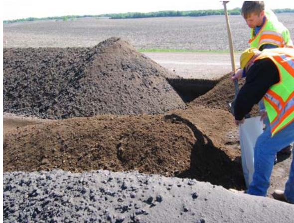
Figure 2.1: RAP, Aggregate, and In-situ Blend Produced from County Road (CR) 3.
