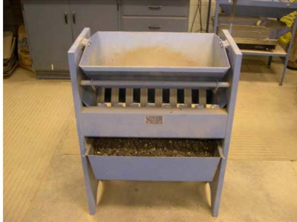
Figure 2.2: Soil Splitter.
