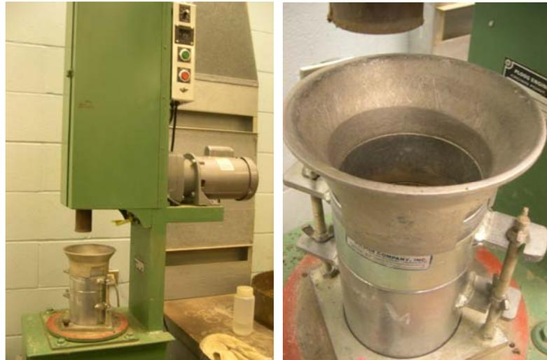
Figure 2.6: Proctor Compaction Test Hammer and Mold.
