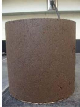
Figure 2.8: Gyratory Compacted Specimen.
