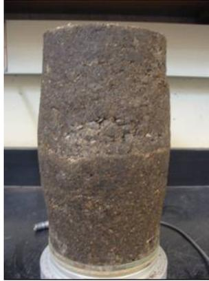
Figure 2.20: Specimen Compacted by Gyratory Compactor After Strength Testing.
