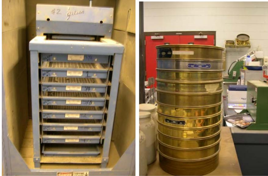
Figure 2.3: Sieves for Coarse Grained Soil (Left) and Fine Grained Soil (Right).
