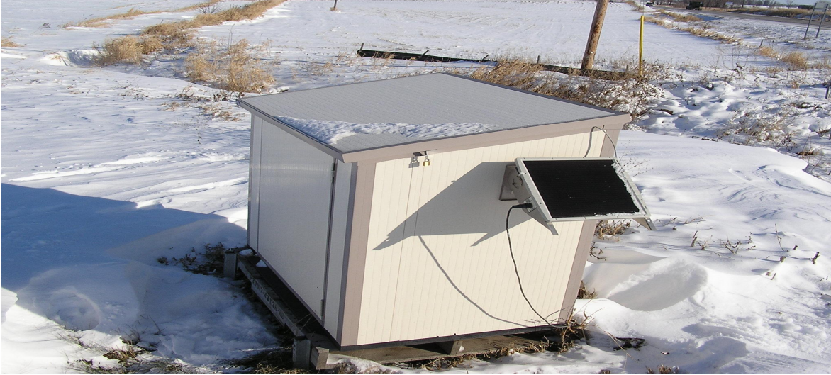
Figure 3.17: Wooden environmental cabinet & solar panel at the outlet of Carver County dry detention pond
