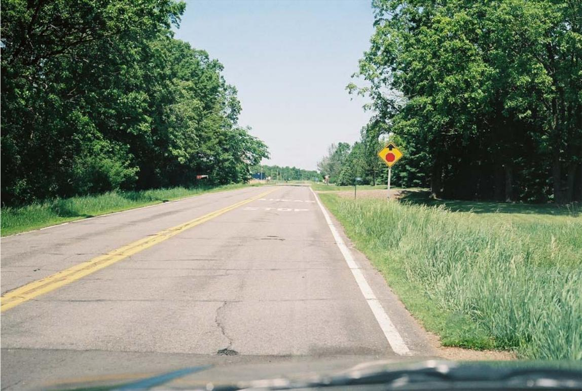
Photograph #218 (Reel #11, 4A) (from South, looking North): first rumble strip *missing* (because of new road surface) but warning sign in view and STOP AHEAD visible on road.
