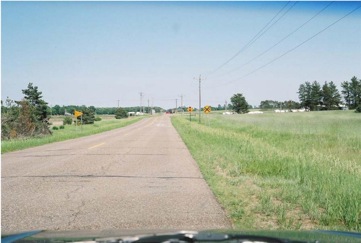
Photograph #263 (Reel #13, 1) (from West, looking East): first rumble strip is filled in (as are second rumble strips; warning sign in view; also, rail crossing sign in view and STOP AHEAD on road.
