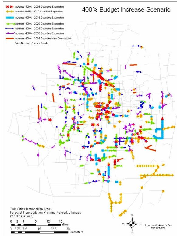
Computer modeling was used to generate different highway network scenarios given different construction decision rules and investment levels.
