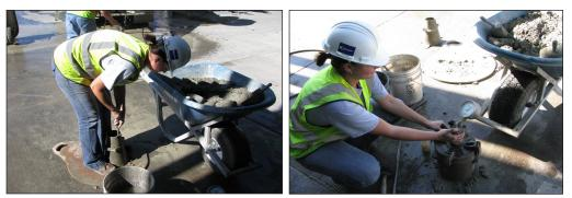
Researchers measured workability using the slump test (left), in which an inverted cone-shaped mold is removed from soft concrete and the resulting slumping measured. They measured plastic air content by using a pressure gauge (right) to calculate the percentage of the soft mixture composed of air bubbles.
