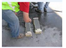
Researchers cast and cured concrete samples to test hardened air content, compressive strength and freeze-thaw durability.
