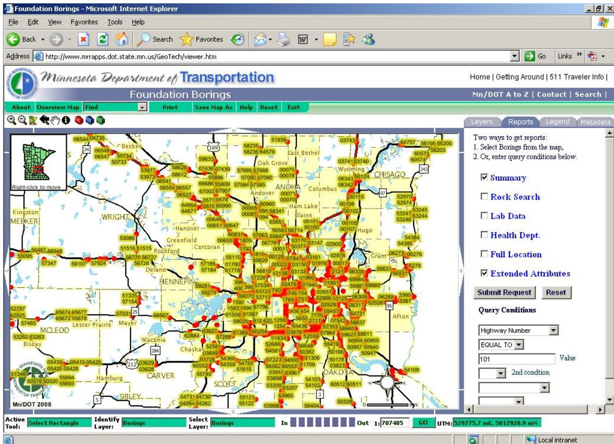
**Figure 1.1** The second generation Foundations Boring website. Users could navigate to locations of interest using pan and zoom commands, as well as execute queries to generate reports listing borehole attributes in 5 predesignated formats.
