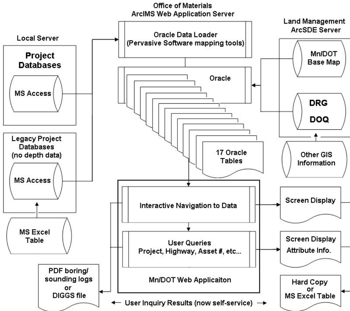
**Figure 1.3 Diagram of the new MnDOT Foundation Boring ArcGIS application.**
