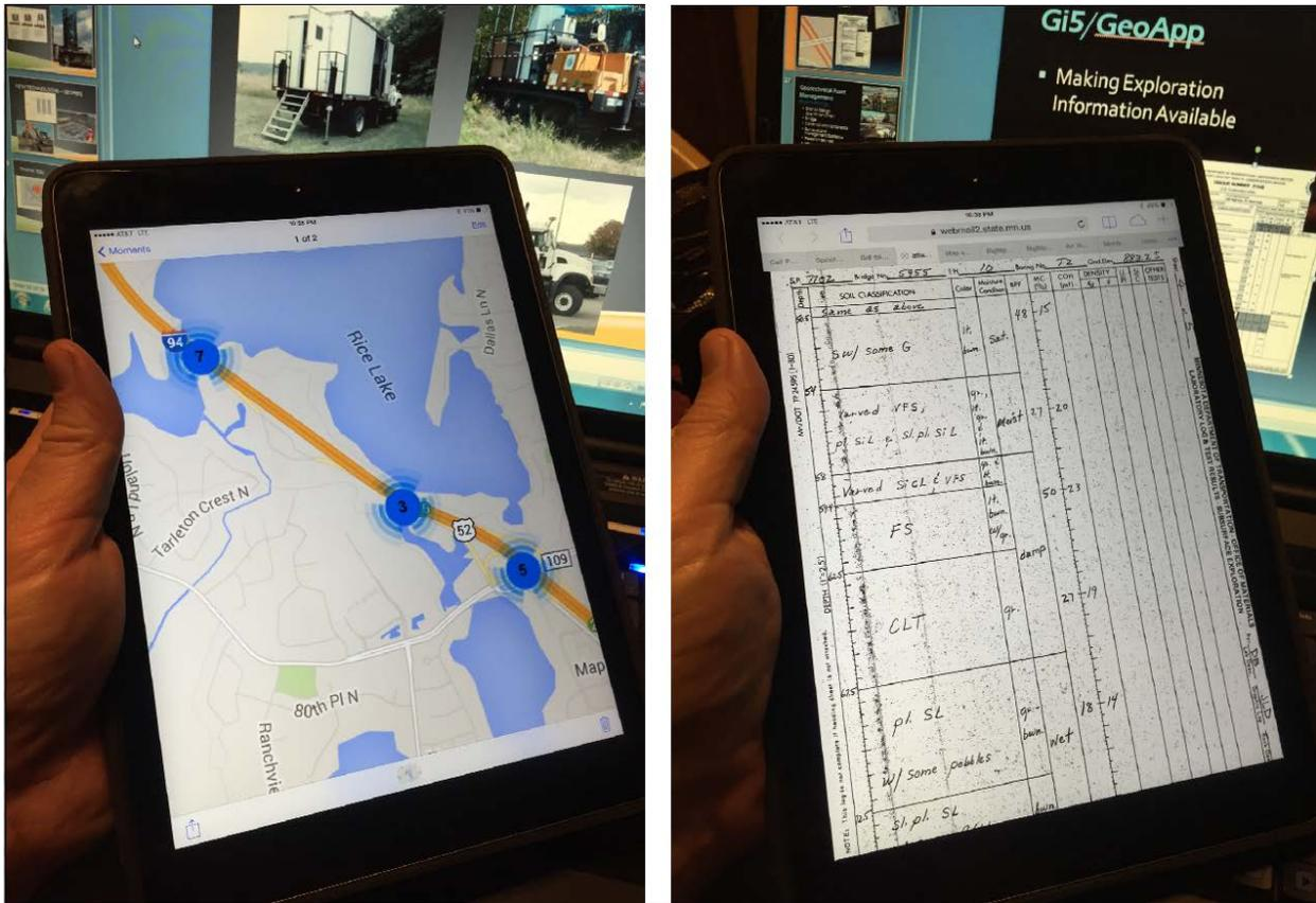
*Figure 6.1 The GeoApp allows the functionality of the desktop Gi5 application tailored to mobile devices to make use of the touch-screen and GPS functionality.*
