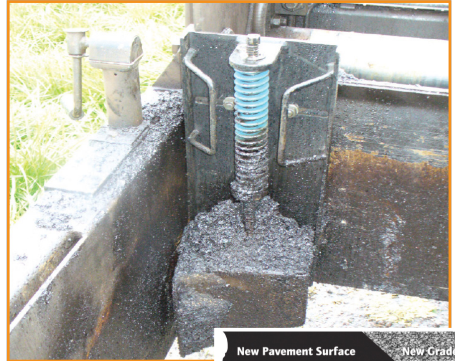
The shoe that creates the safety edge
