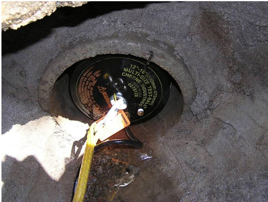
**Figure C.13:** 12” diameter inflatable plug loaned by the City of St. Louis Park Public Works for use at CBMH4 as shown in Figure C.12.
