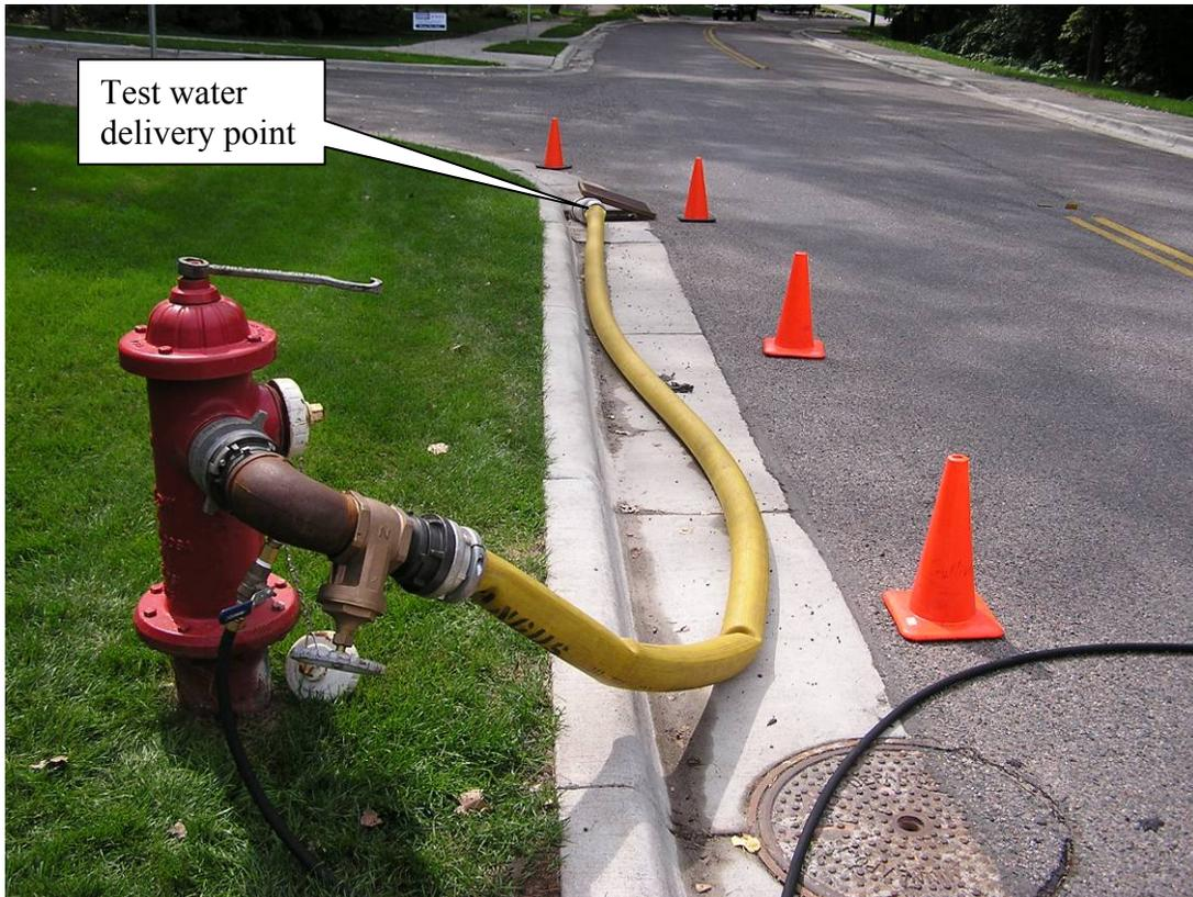
**Figure C.24:** Influent piping system from hydrant to catch basin for CDS testing.
