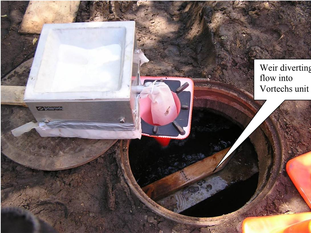
**Figure C.15:** Sediment feeding location at STMH3B.
