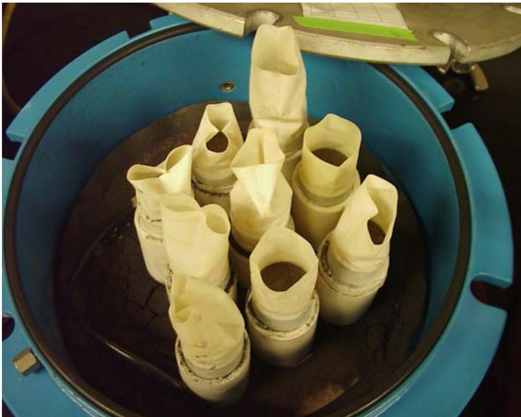
**Figure 6: Molded soil specimens with rubber sleeves on the pressure plate in a pressure chamber. The pressure chamber was used to bring specimens to a given soil suction.**
