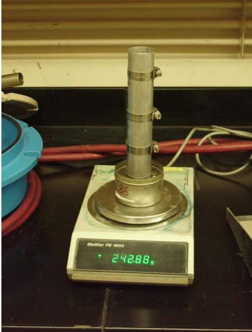
**Figure 5: Split mold used to construct specimens. Mold diameter was 3.81 cm.**
