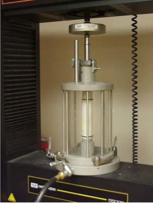
**Figure 7: Equilibrated soil specimen ready for shearing in a triaxial cell.**
