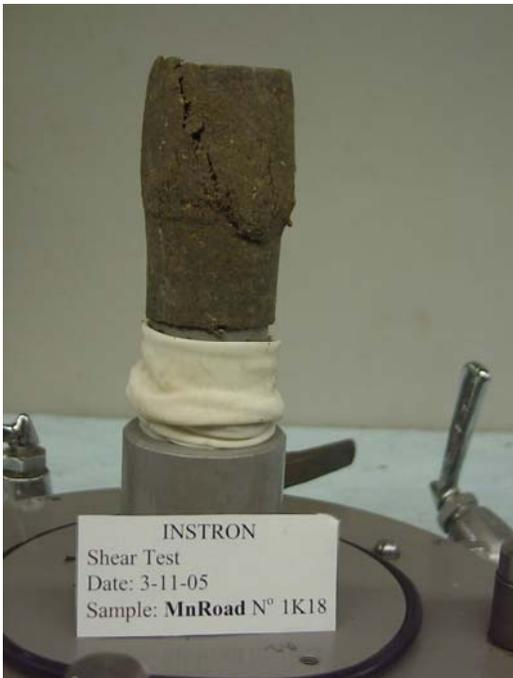
**Figure 8: Sheared soil specimen.**
