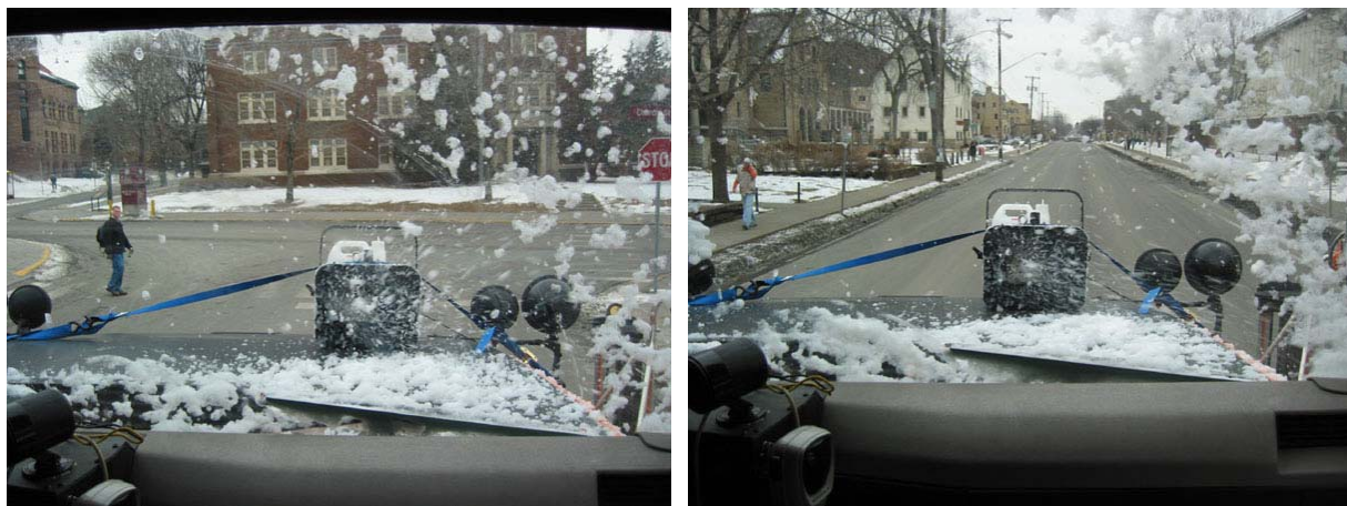
Figure A-2. Foam-snow machine during pilot testing on the hood of a plow truck
