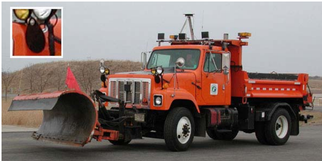
Figure 2.2. The truck equipped with a front plow and the DAS that was used during track testing and (insert) close-up of right headlight blinder while not covering light
