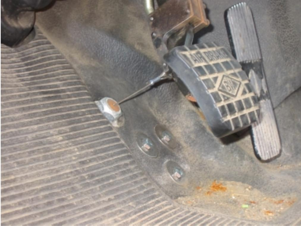
**Figure 5-7: Cable runs through firewall and attaches to brake pedal.**
