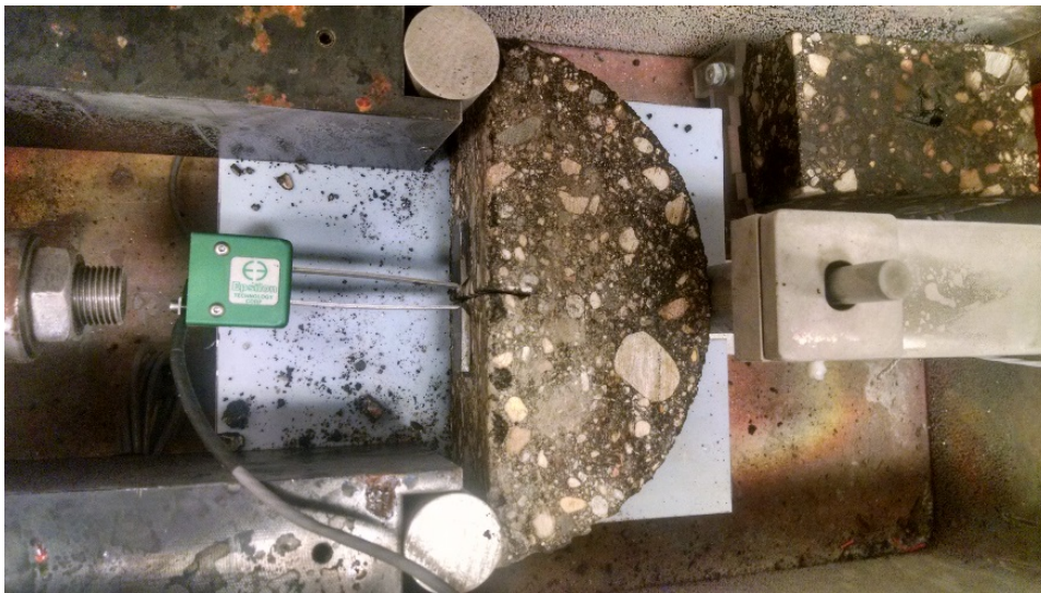
Figure 3.3 CMOD gauge mounted on SCB sample
