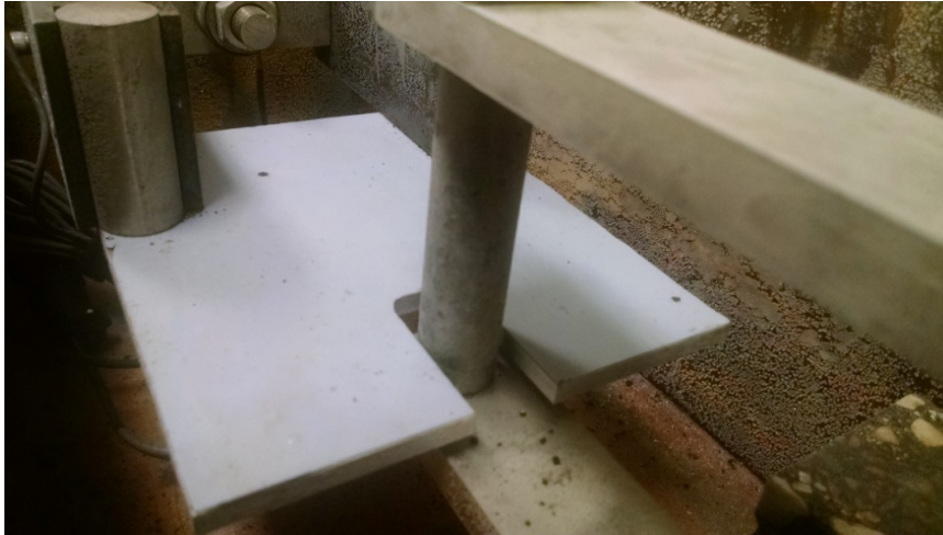
Figure 4.3 Aluminum bottom plate covered with Teflon strip in horizontal setup
