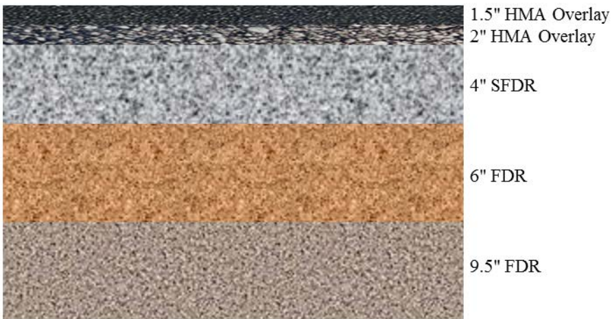
Figure 4. Schematic illustration of pavement structure for Beltrami County CSAH 36
