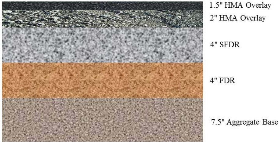
Figure 2. Schematic illustration of pavement structure for Beltrami County CSAH 5
