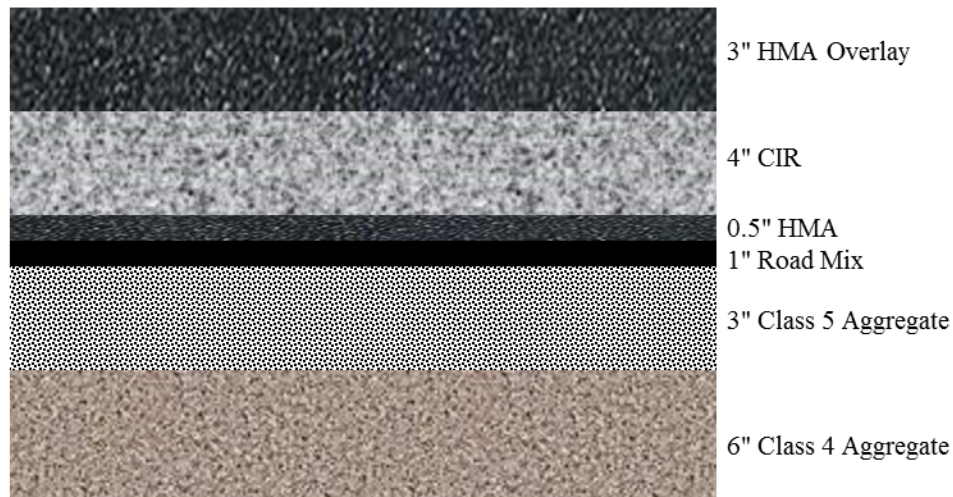
Figure 9. Pavement structure for Brown County CSAH 23
