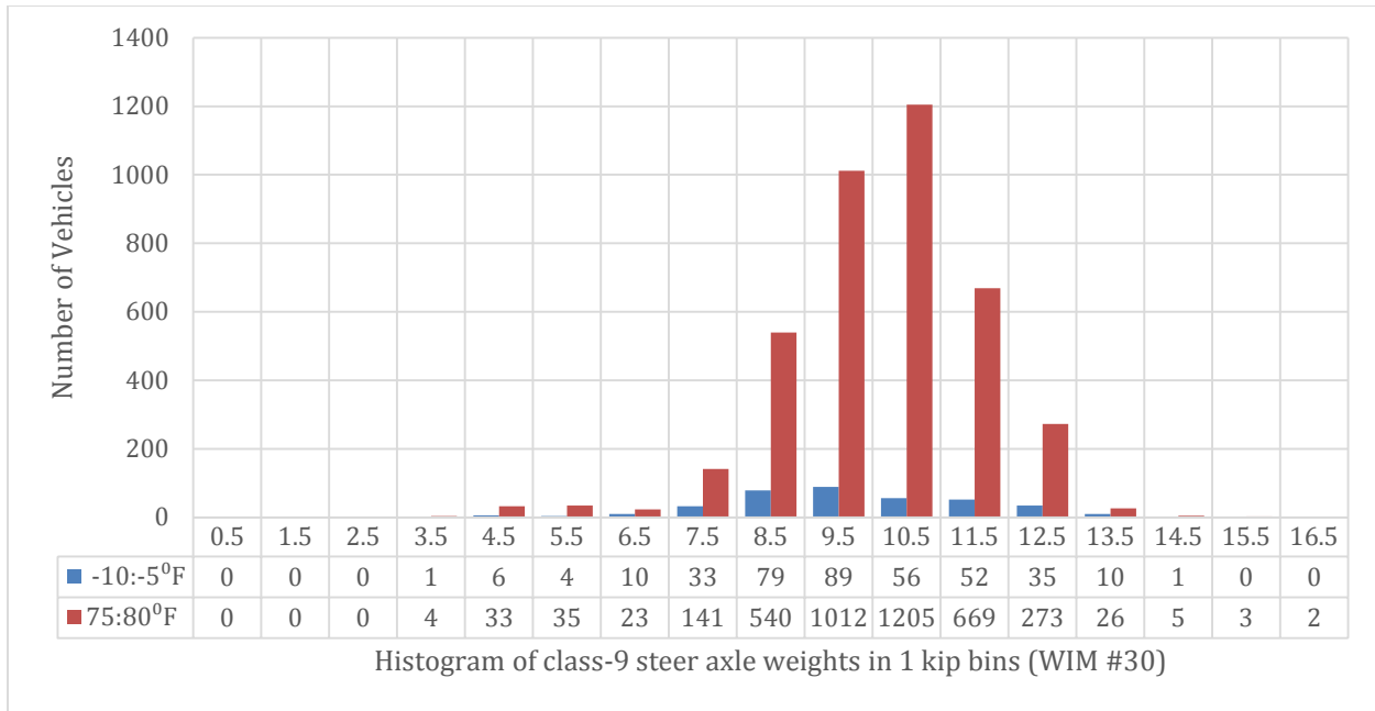
Figure 3.12: Histogram of class-9 steer axle weights of WIM #30 site in two different temperature ranges, after temperature-based calibration
