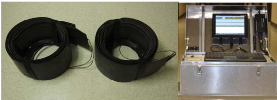
Figure 1: Components of a PWIM System: A Pair of Weigh-Pads and the PWIM Controller
