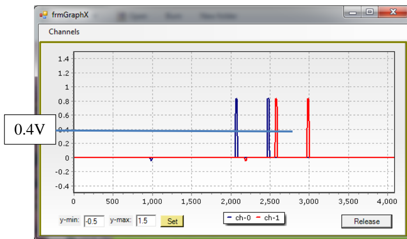
Figure 16: Signal Threshold Measurement Screen
