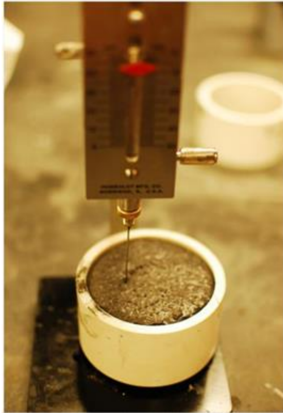
Figure 2.11. Humboldt Vicat needle used for initial Rapid Patch set time tests.
