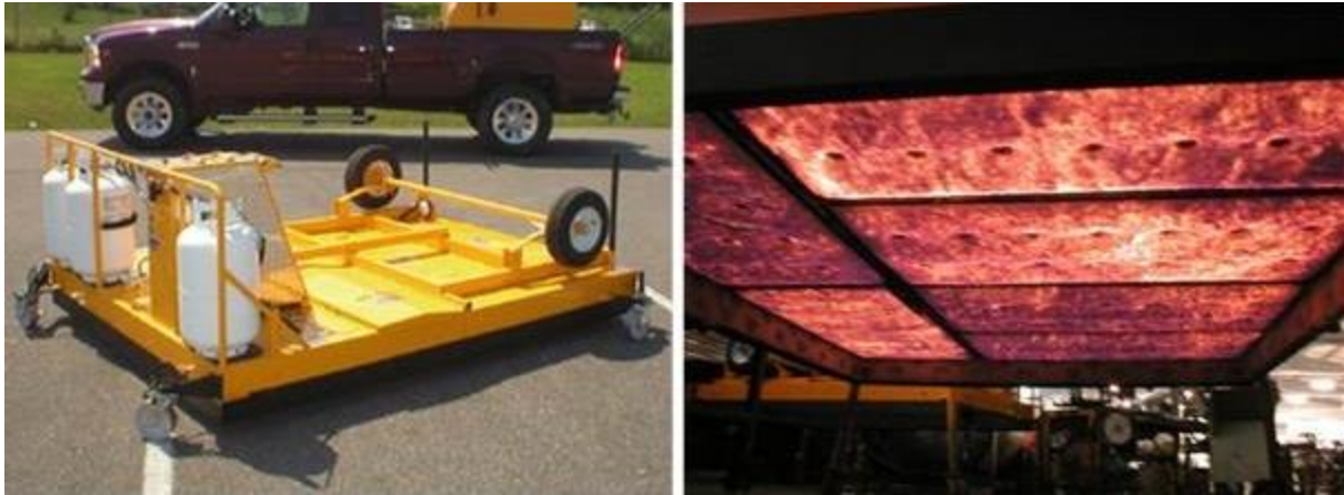
Figure 2.5. Infrared heater (left) and its heating elements (right). (Source: http://www.surelineinc.com/asphalt.html )
