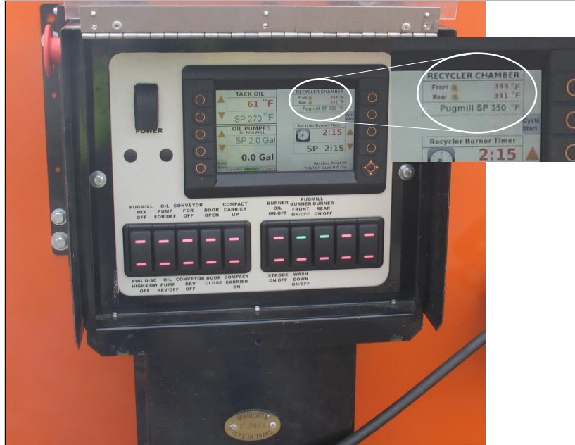
Figure 3.9. Stepp controls, showing recyler chamber temperature (341° F to 344° F).
