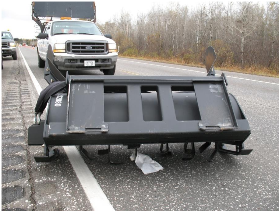
Figure 3.4. "Roto-tiller" attachment for HeatWurx.
