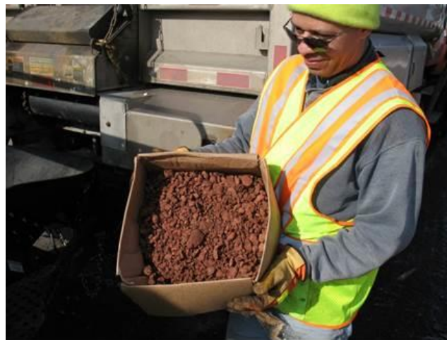
Figure 3.10. Asphaltic additives used with Stepp recycler.
