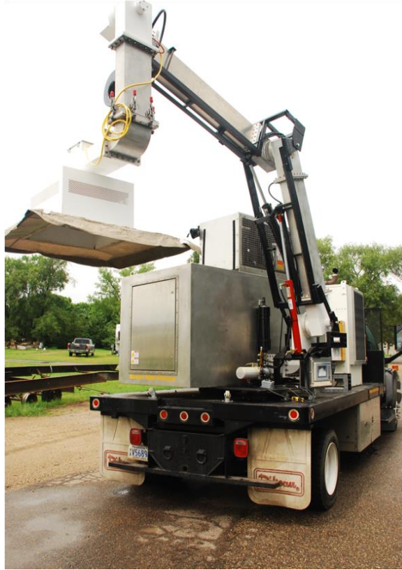
Figure 2.7. Microwave unit with articulating arm.
