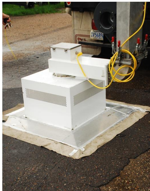
Figure 2.8. Microwave horn and shielding.
