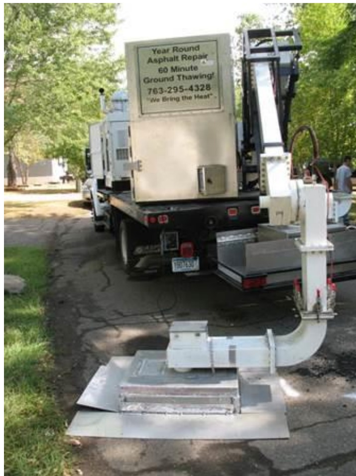
Figure 3.77. Modified microwave equipment: September 10, 2013 field test, Monticello, MN.
