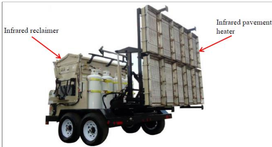
Figure 2.4. Tow-behind combination infrared asphalt heater/reclaimer. (Source: Nazzal et al., 2014)
