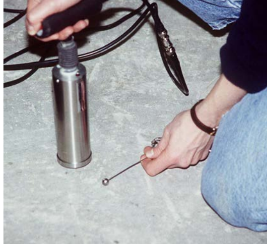
Figure 16: Impact echo setup with a steel ball mounted on a steel spring rod (Carino, 2001).
