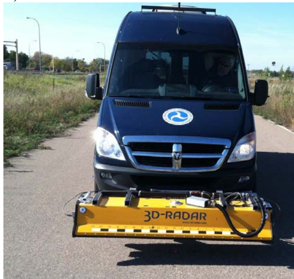
Figure 14: Air coupled step-frequency GPR mounted on a van for high speed measurements.
