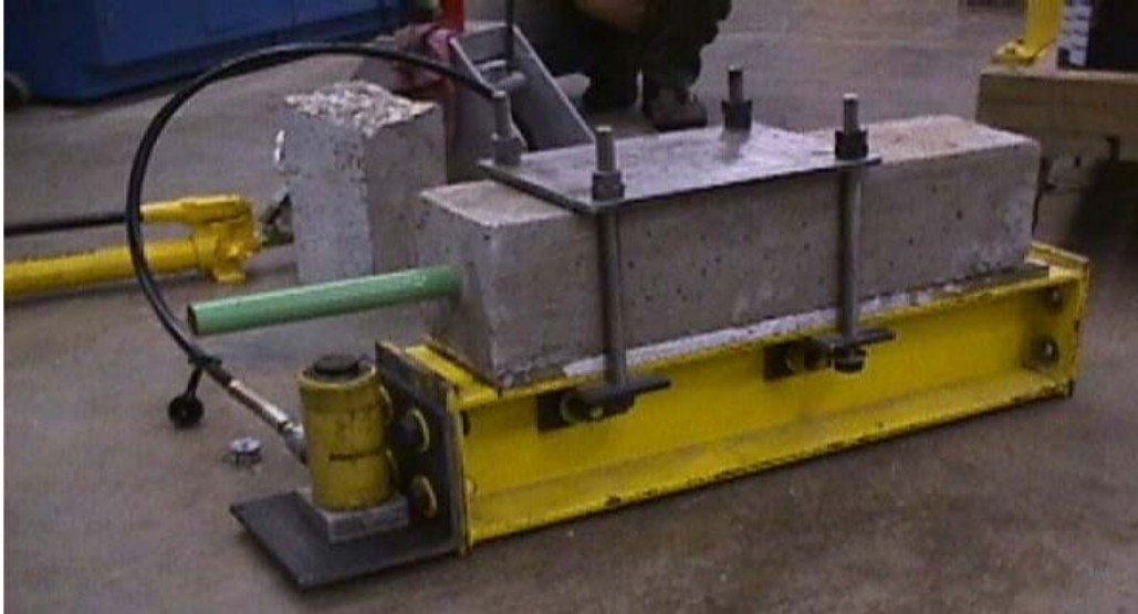
Figure 5: Exposed dowel test specimen.
