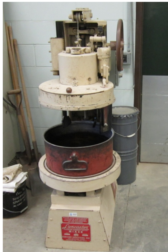
Figure 7: Bituminous Design Mixer
