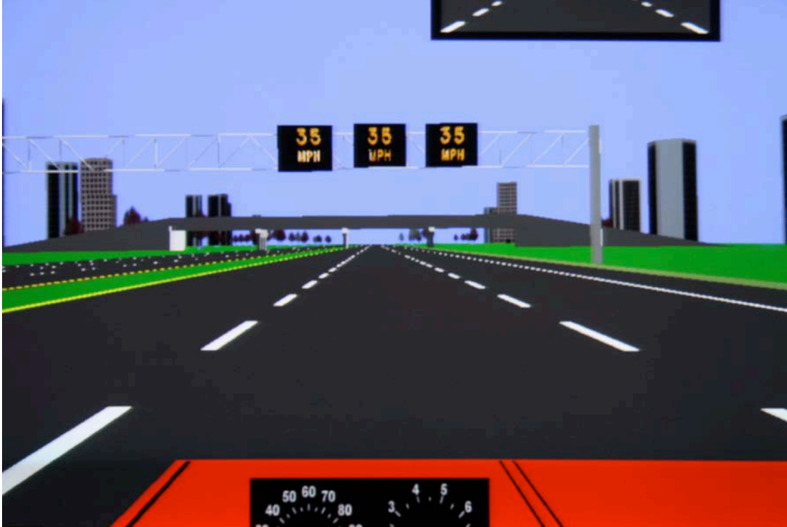
Figure 2.3 The second set of ILCSs displaying the 35-mph speed limit
