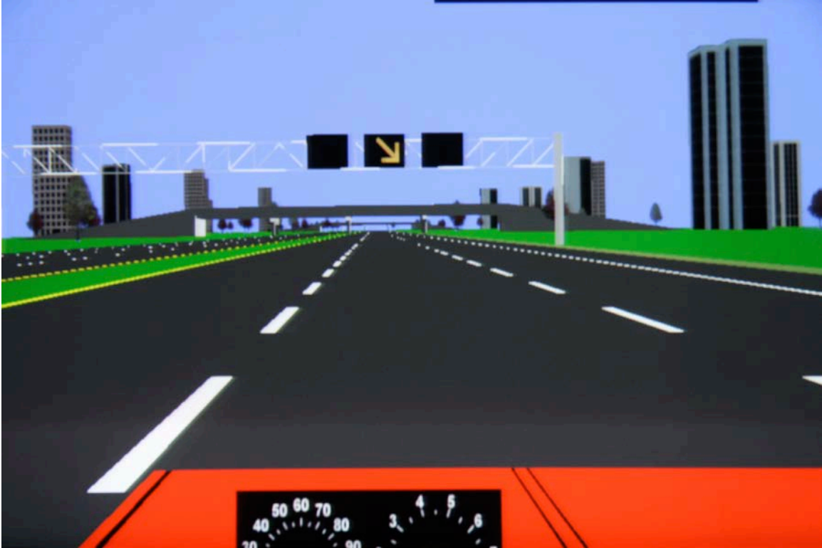
Figure 2.5 The fourth set of ILCSs with a diagonal arrow indicating merge right
