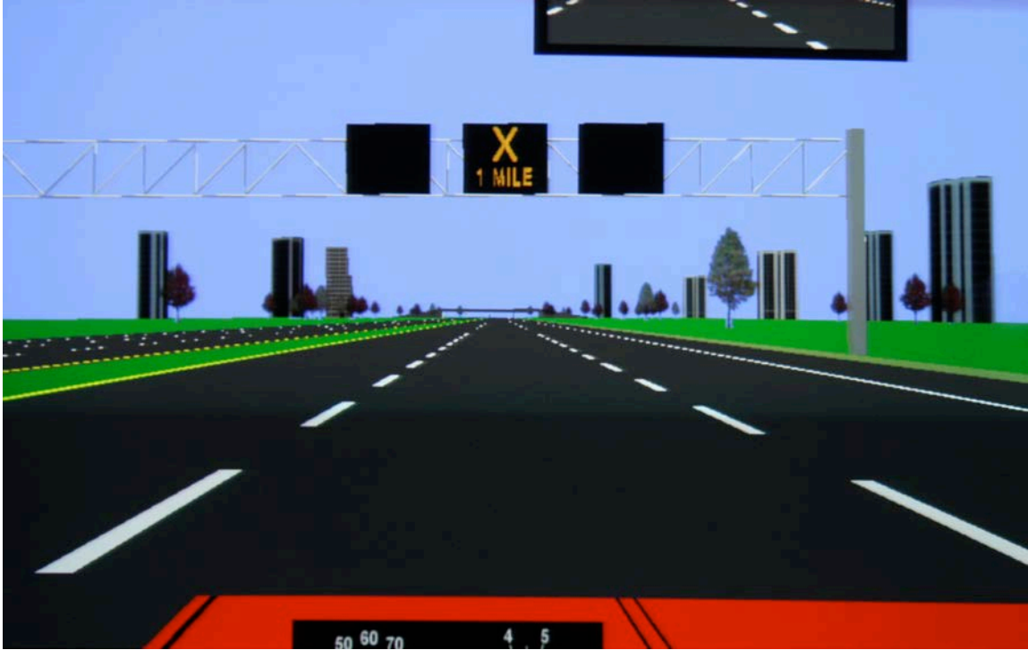
Figure 2.4 The third set of ILCSs with the “X/1 mile” lane closure warning on the center display
