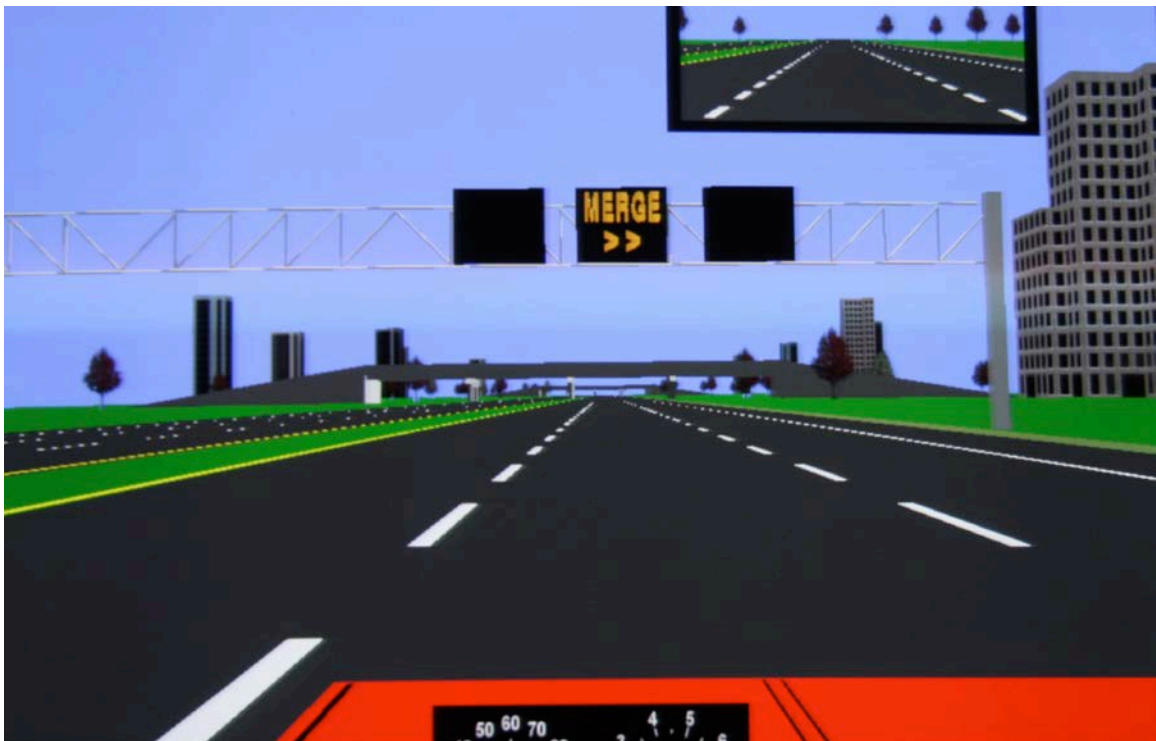
Figure 2.8 The fourth set of ILCSs with the second in the sequence of dynamic chevrons indicating merge right
