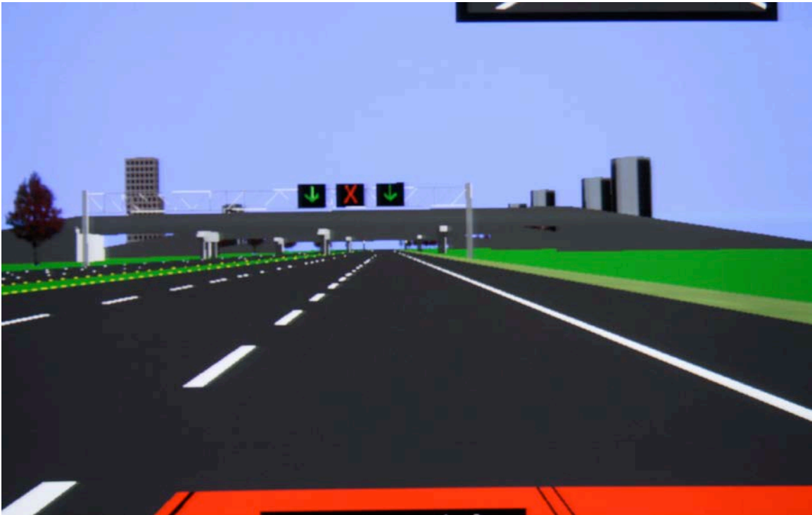
Figure 2.10 The fifth set of ILCSs with the “X/1 mile” lane closure warning on the center display and green arrows on the left and right ILCSs
