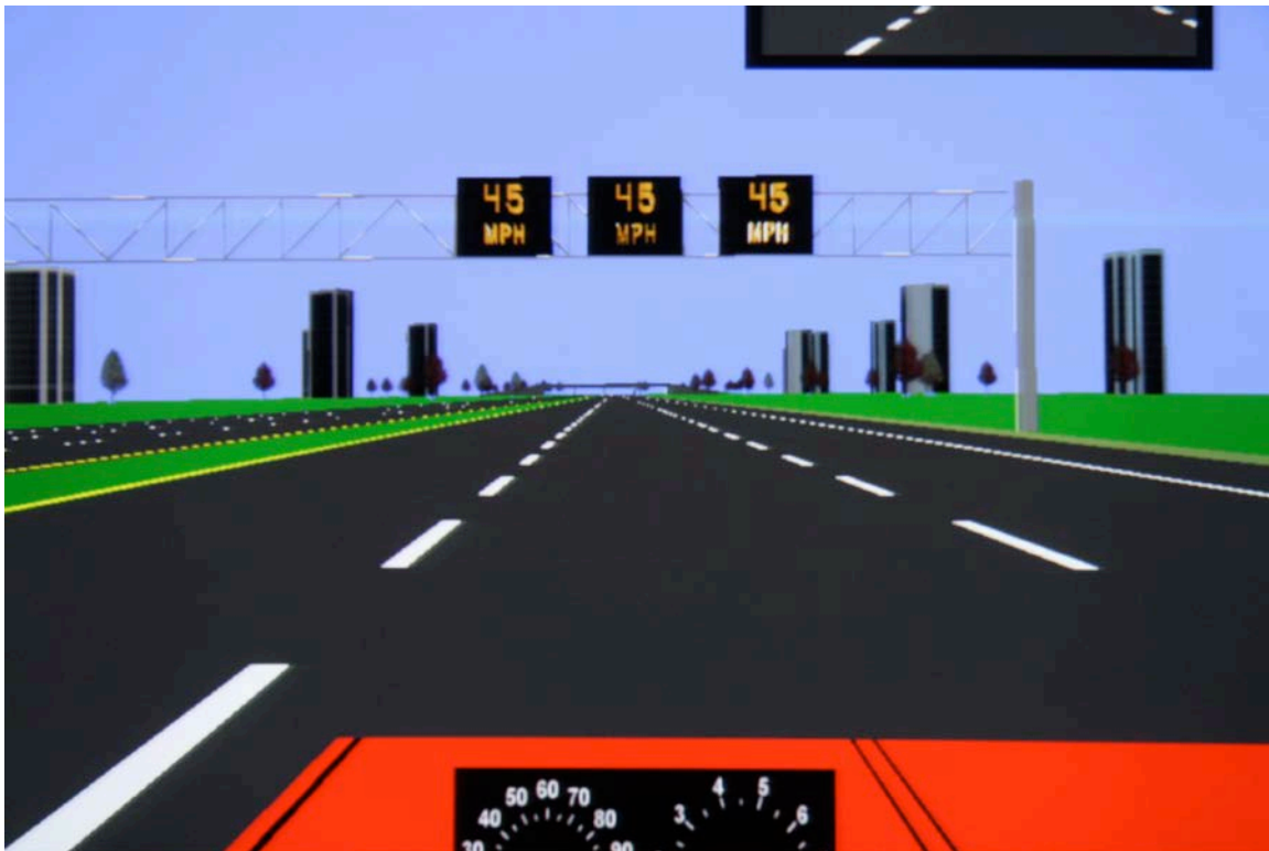
Figure 2.2 The first set of ILCSs displaying the 45-mph speed limit
