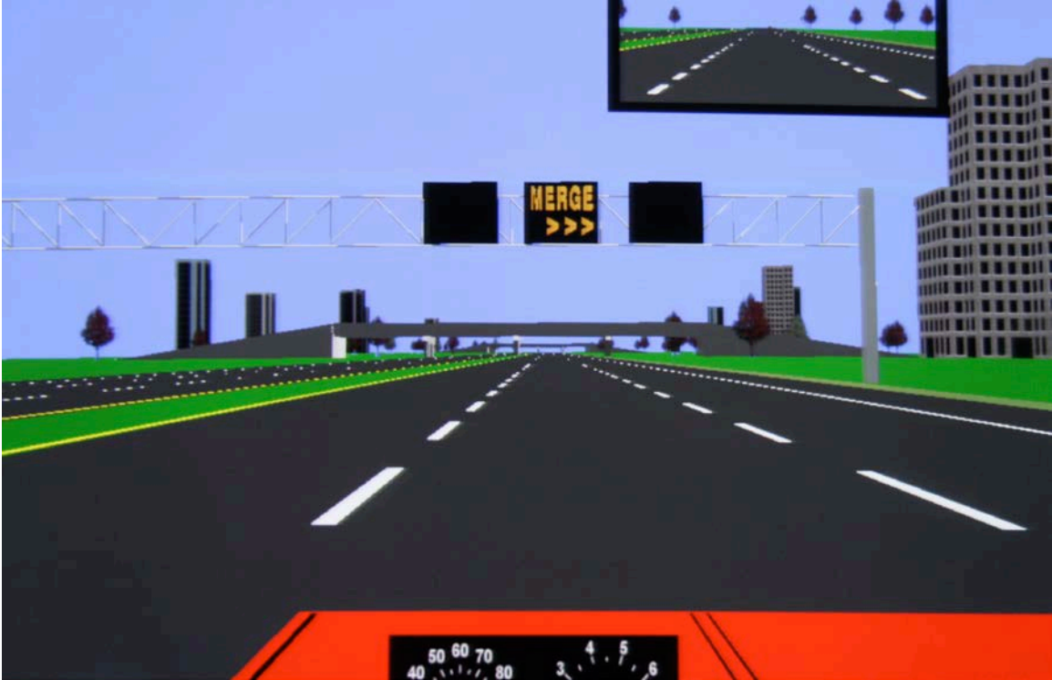
Figure 2.9 The fourth set of ILCSs with the third in the sequence of dynamic chevrons indicating merge right
