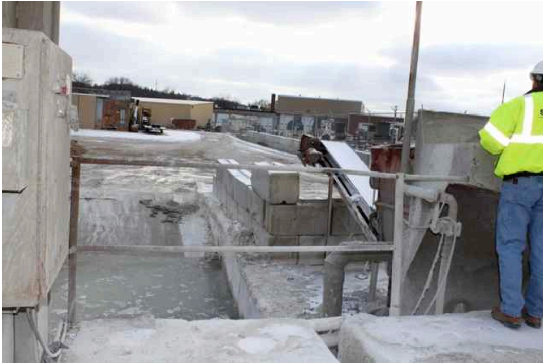
Figure 2: Truck washout discharge station, with desander screen and conveyor.
