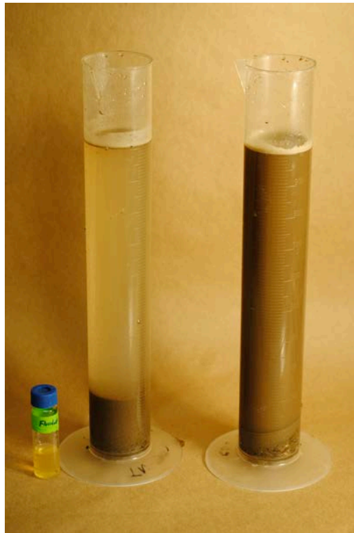
Figure 4 Effect of flocculent addition (left), approximately 90 seconds after flocculent addition and mixing to a solution of Minnesota River silt in water.
