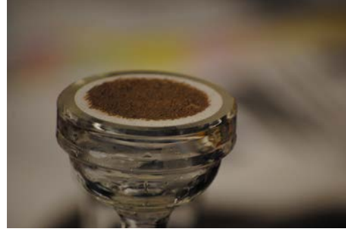
Figure 14 Geotextile filter removal of 1 g of bridge deck debris sediments in 100 mL of water through a 47 mm diameter glass filter apparatus. Left: coarser sediments retained by a rock bag woven geotextile, view down into the filter cone prior to disassembly. Right: finer sediments retained by a 0.45 um glass fiber filter from beneath the rock bag woven geotextile.
