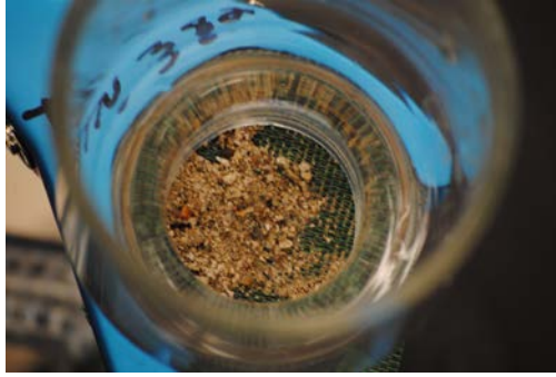
Figure 14 Geotextile filter removal of 1 g of bridge deck debris sediments in 100 mL of water through a 47 mm diameter glass filter apparatus. Left: coarser sediments retained by a rock bag woven geotextile, view down into the filter cone prior to disassembly. Right: finer sediments retained by a 0.45 um glass fiber filter from beneath the rock bag woven geotextile.
