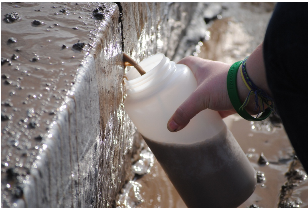
Figure 3: Sampling of saw cut slurry directly after completed cut with flow indicative of maximum generated from cut. Samples taken here later settled and cured into 1" thick coalesced specimen with moderate structural strength.
