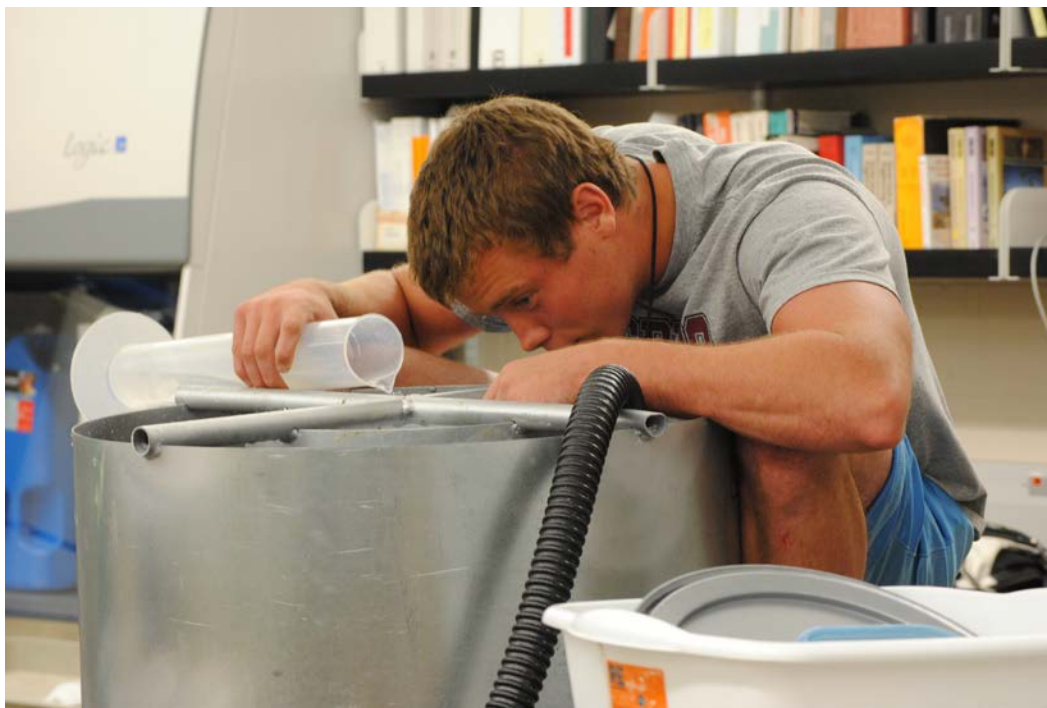
Figure 5 Infiltration testing of sand filter challenged by sediments, using a known volume of water to keep a constant head condition.
