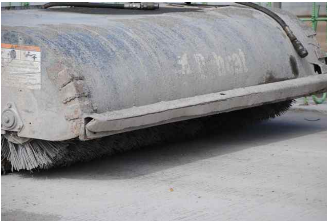
Figure 5: Sweeper for concrete pavement grinding fines management (parked).
