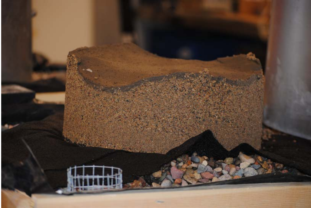
Figure 6 Sand filter layer clogged by pavement grinding sediments.
