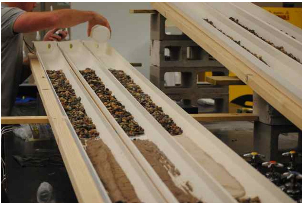
Figure 3 Stream flow bed erosion test apparatus, 0.5 feet per second velocity apparatus on left and 1.0 feet per second velocity apparatus on right. Note use of washed gravel up and down stream of sediment to prevent potential laminar flow conditions.
