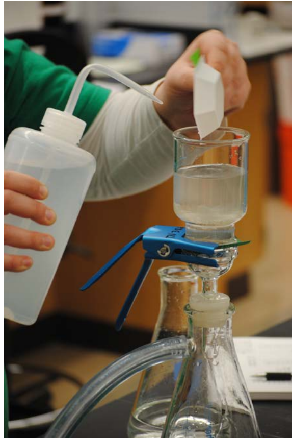
Figure 13 Deionized water stream being used to rinse all sediment from weigh dish during geotextile filter removal of approximately 1 g of bridge deck debris sediments in 100 mL of water through a 47 mm diameter glass filter apparatus with a rock bag woven geotextile above a 0.45 \mu m glass fiber filter.
