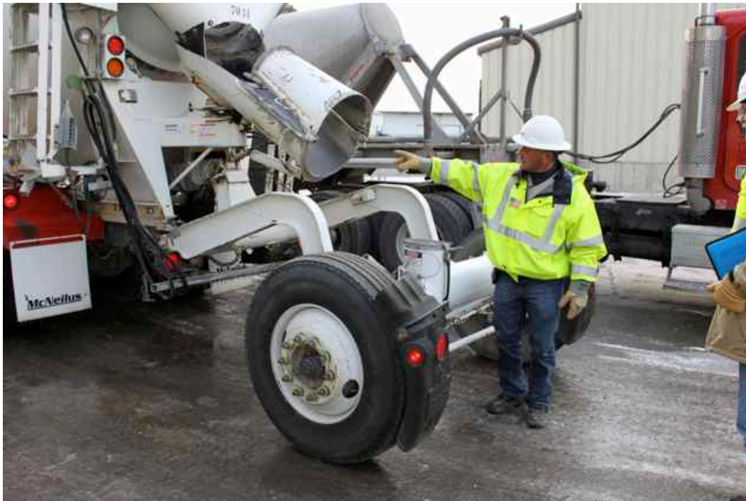
Figure 1: Ready mix truck with pony axle-mounted wash water capture tank that drains back to mixer upon raising.
