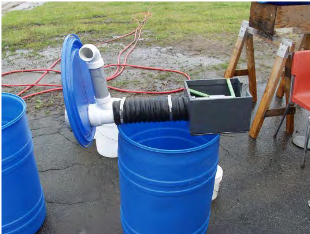
Figure 4.12. Collection tank with flow meter
