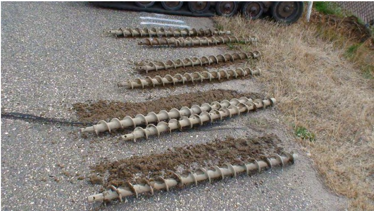
Figure 1.5. Well #2: Saturated sands at up to 30-foot depths
