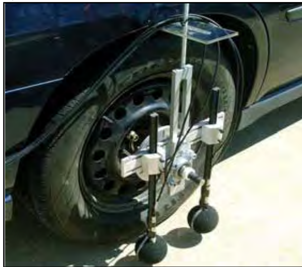
Figure 5.43. MnDOT on-board sound intensity microphones
