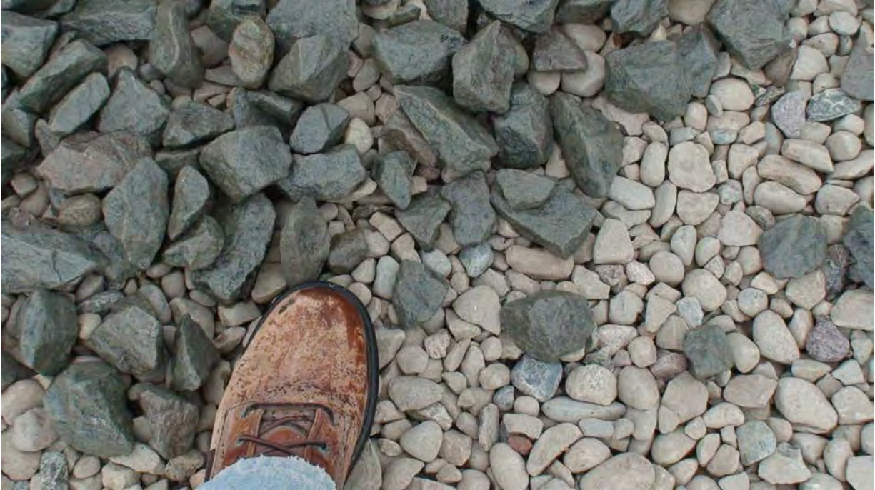
Figure 4.5. Railroad ballast / CA-15 composite base
