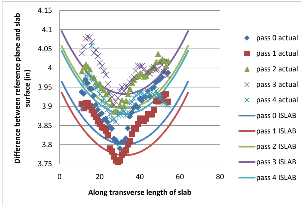
Figure 148: Cell 12 actual data and ISLAB2000 curve from the 5th order polynomial approximation
