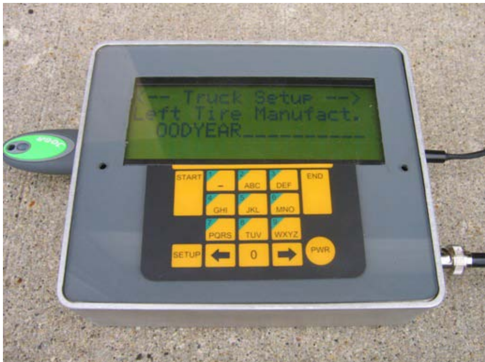
Figure 5.27. Truck Setup Screen 6 for Prototype Test Roller System (Left Tire Manufacturer).
