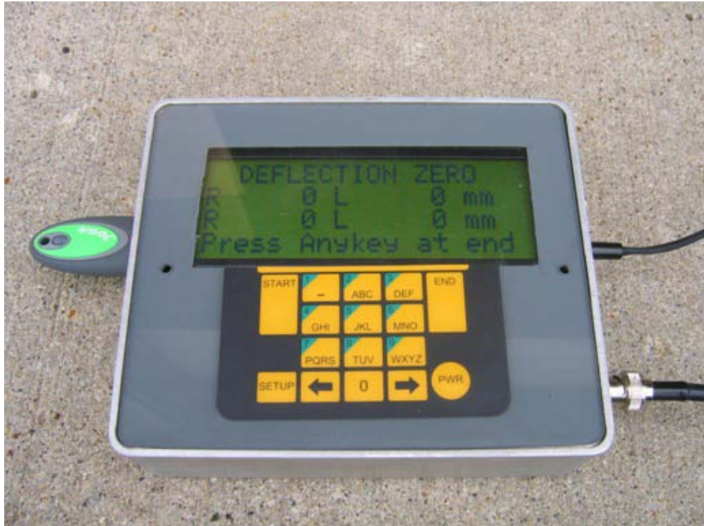
Figure 5.20. Zero Sensors Screen 2 for Prototype Test Roller System (Deflection Zero).
