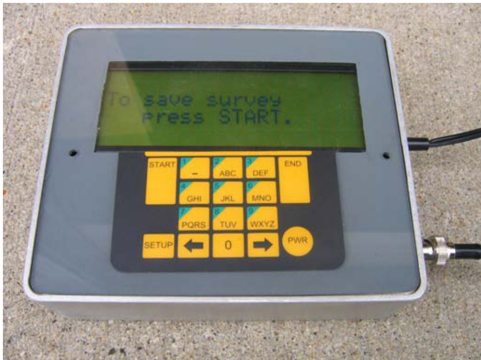
Figure 5.11. Input Screen 10 for Prototype Test Roller System (Save Survey).
