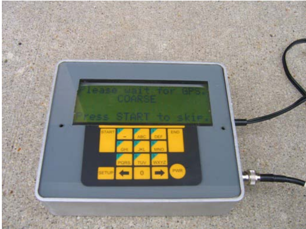
Figure 5.2. Input Screen 1 for Prototype Test Roller System (Wait for GPS).
