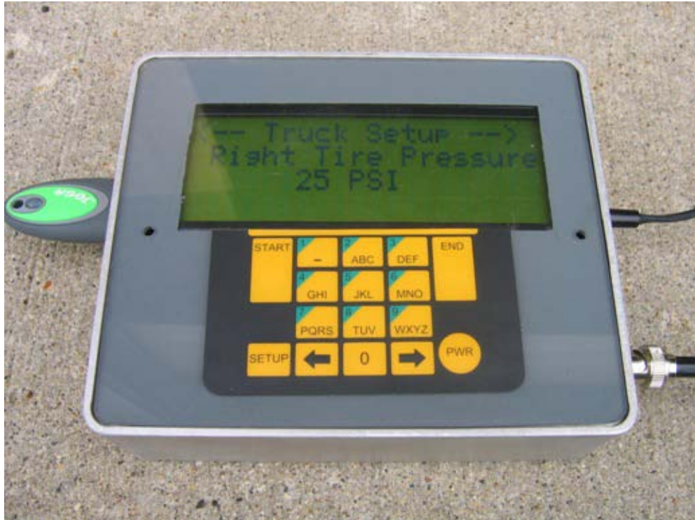
Figure 5.26. Truck Setup Screen 5 for Prototype Test Roller System (Right Tire Pressure).
