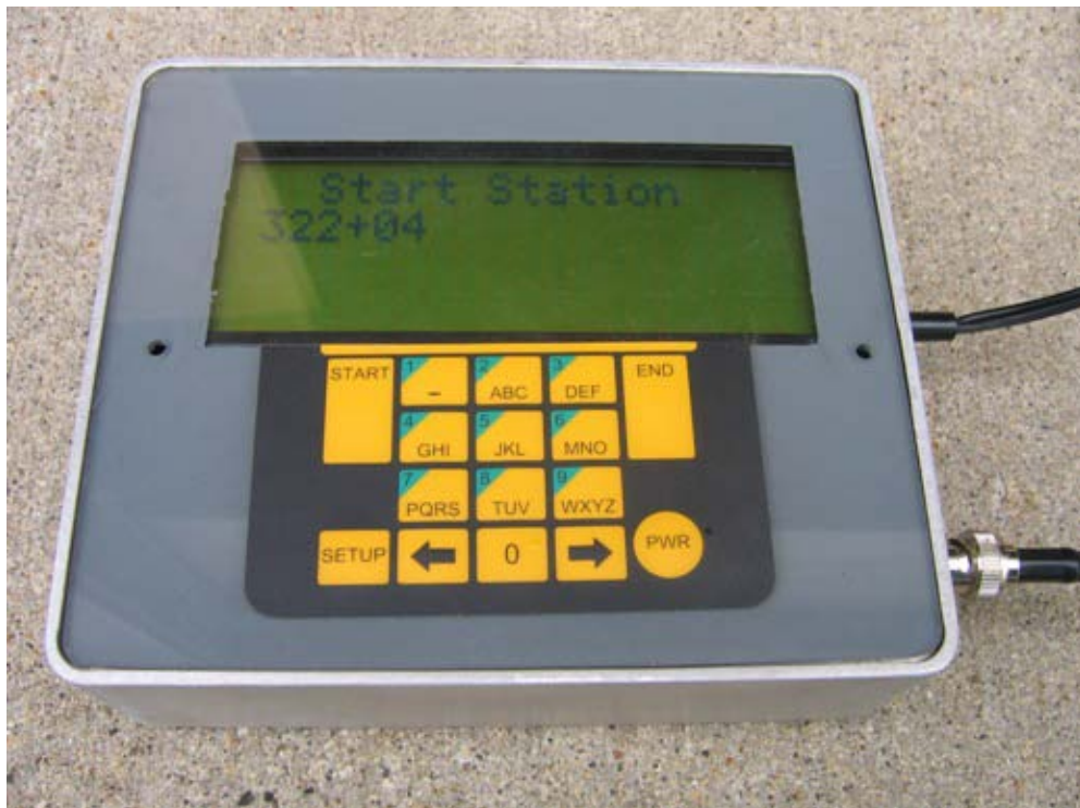
Figure 5.7. Input Screen 6 for Prototype Test Roller System (Start Station).
