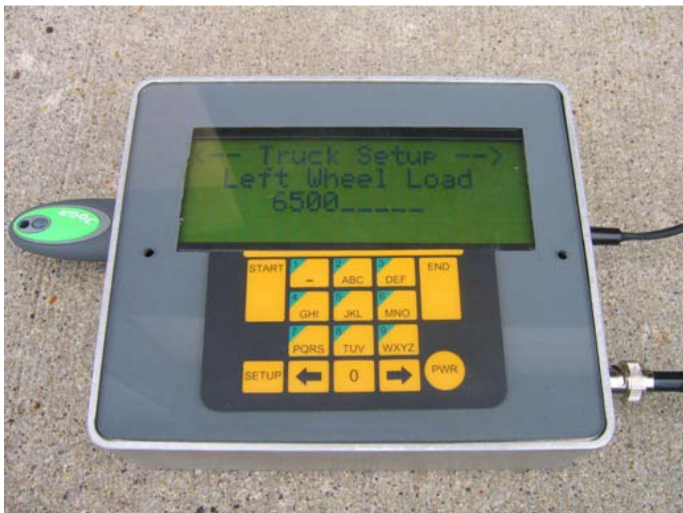
Figure 5.23. Truck Setup Screen 2 for Prototype Test Roller System (Left Wheel Load).
