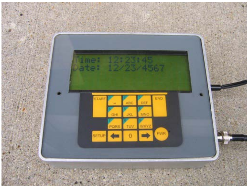
Figure 5.5. Input Screen 4 for Prototype Test Roller System (Timestamp from GPS).
