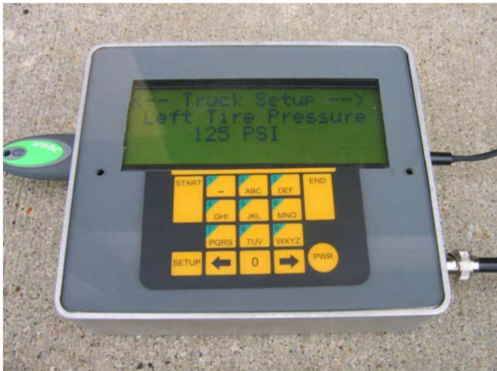
Figure 5.25. Truck Setup Screen 4 for Prototype Test Roller System (Left Tire Pressure).
