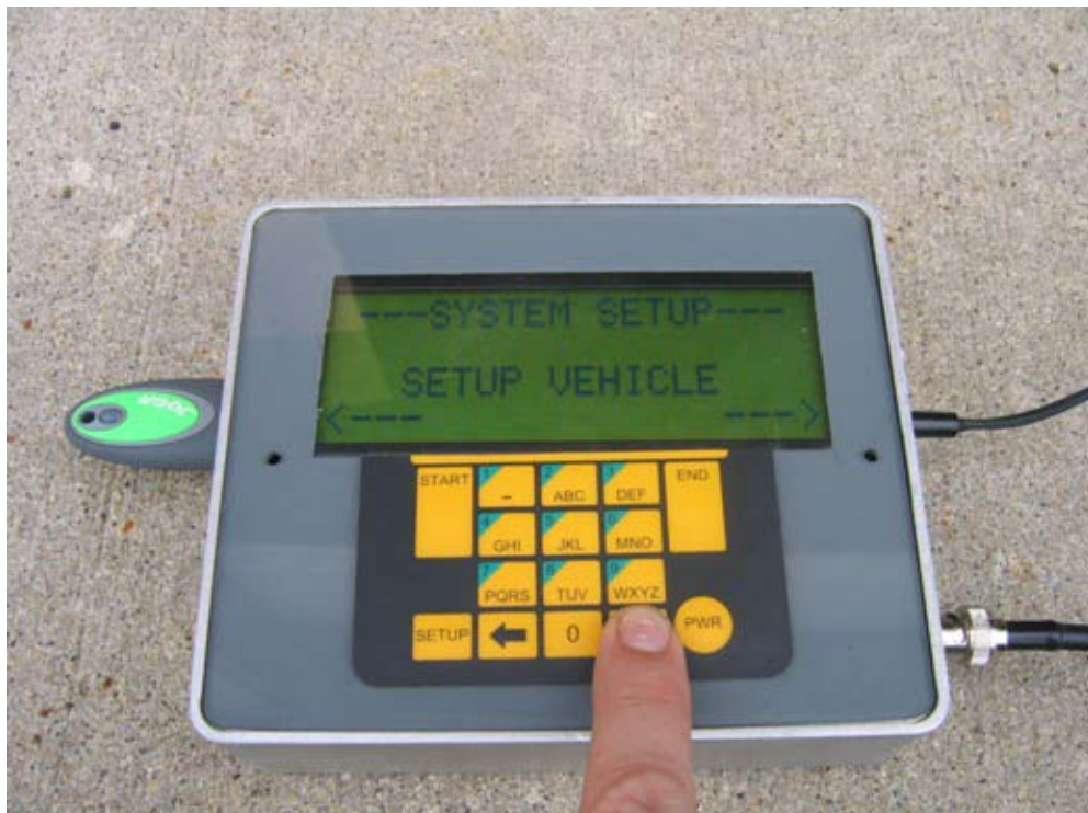
Figure 5.15. System Setup Screen 2 for Prototype Test Roller System (Setup Vehicle).
