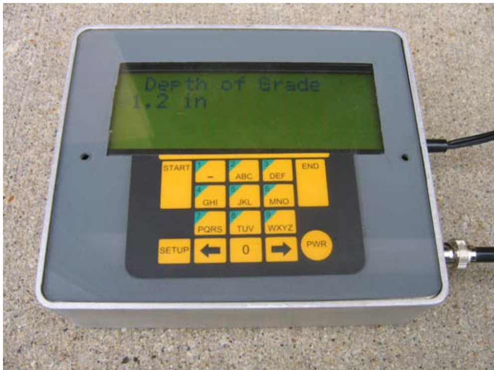
Figure 5.9. Input Screen 8 for Prototype Test Roller System (Depth of Grade).
