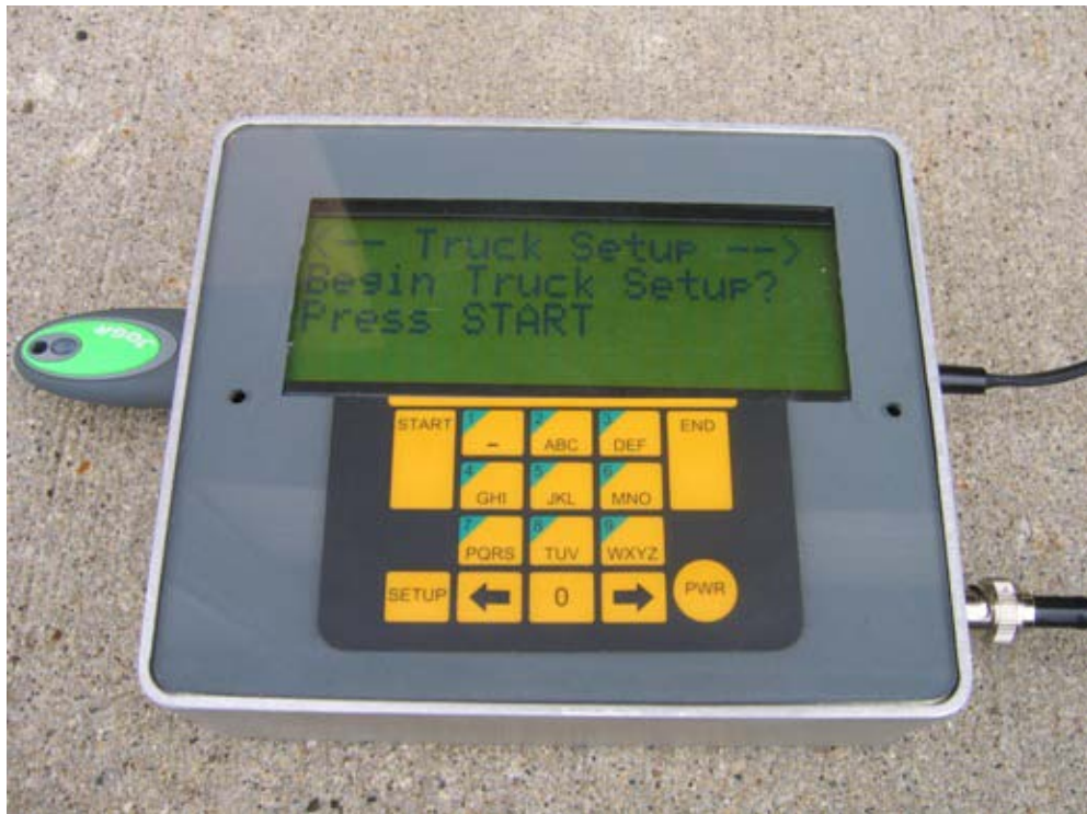
Figure 5.22. Truck Setup Screen 1 for Prototype Test Roller System (Truck Setup Press Start).
