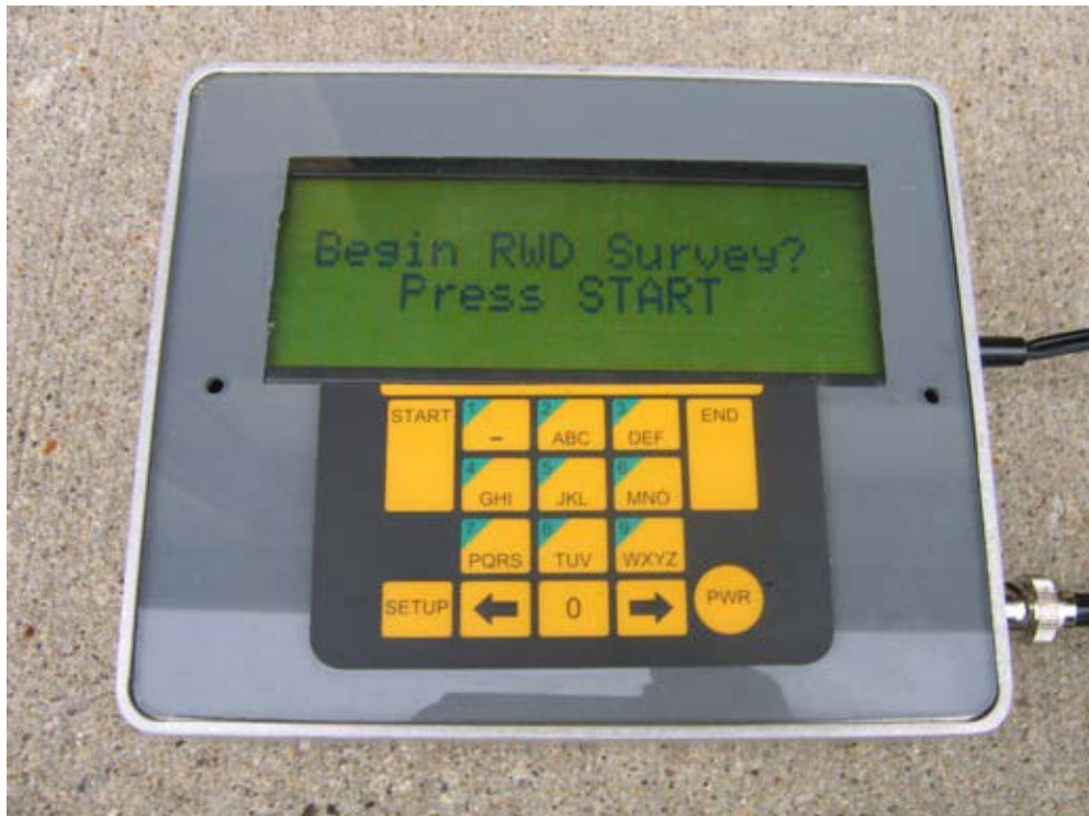
Figure 5.4. Input Screen 3 for Prototype Test Roller System (Begin Survey?).
