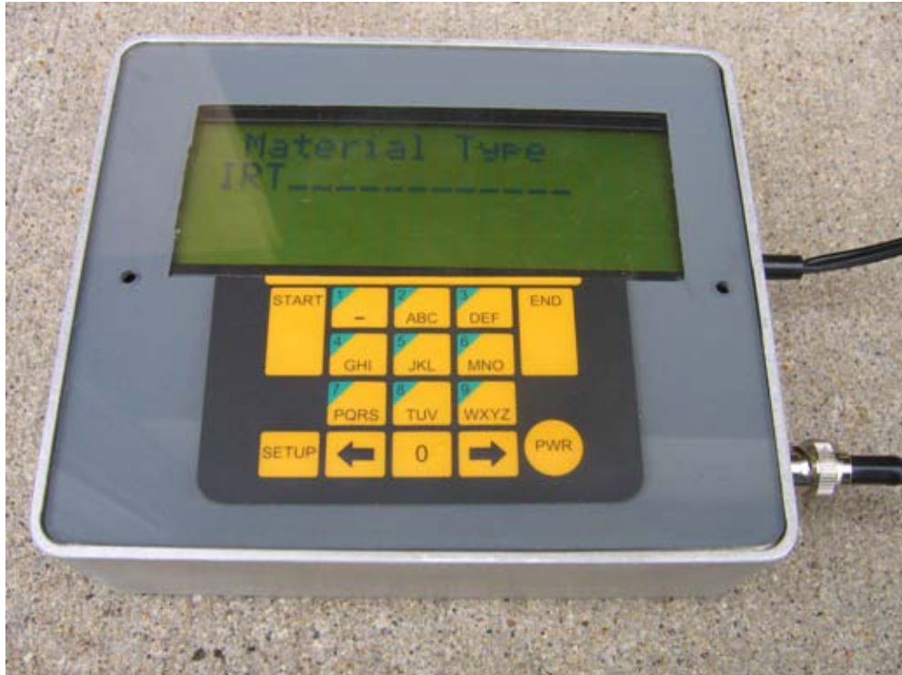
Figure 5.10. Input Screen 9 for Prototype Test Roller System (Material Type).
