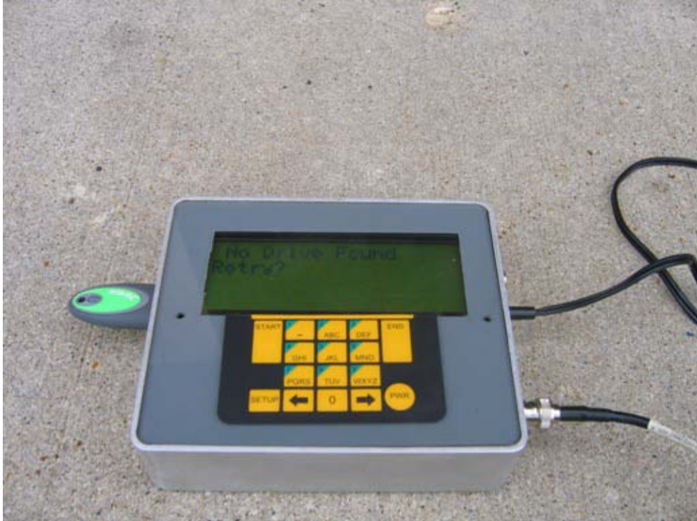
Figure 5.12. Input Screen 11 for Prototype Test Roller System (No USB Drive Warning).
