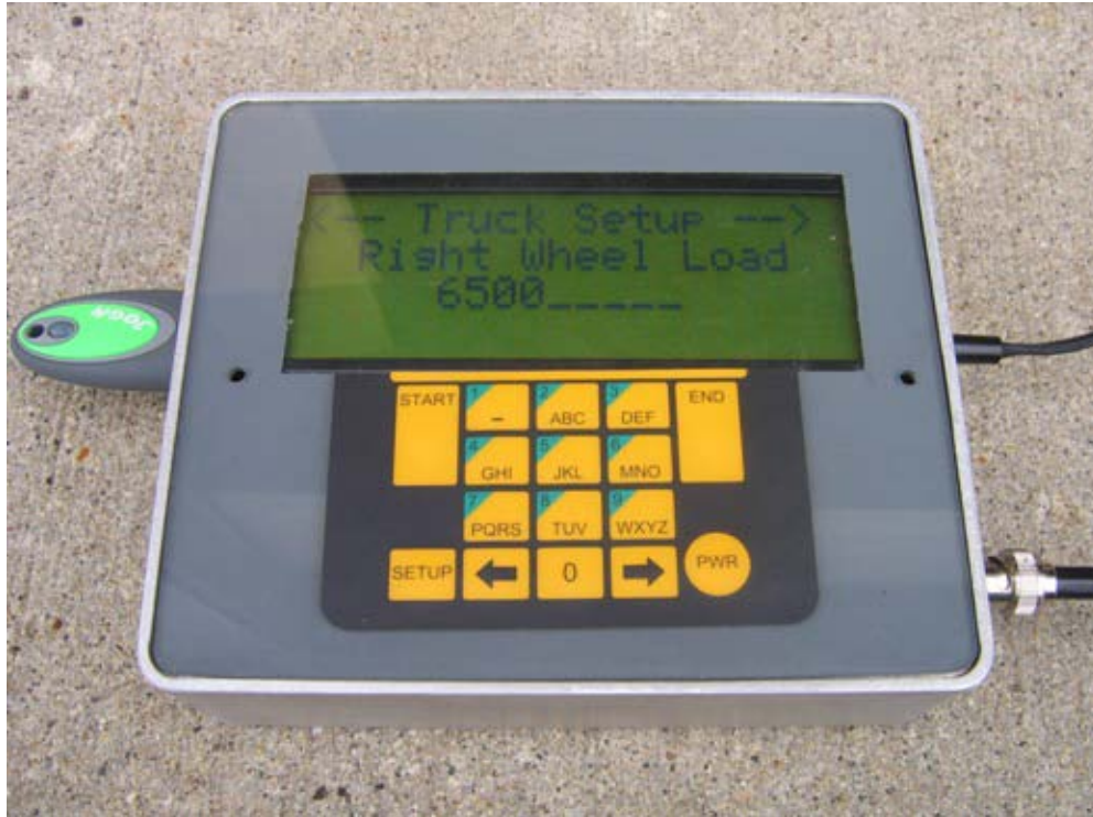
Figure 5.24. Truck Setup Screen 3 for Prototype Test Roller System (Right Wheel Load).
