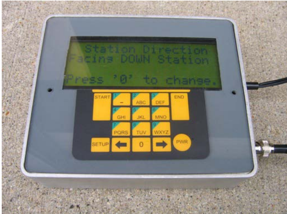
Figure 5.8. Input Screen 7 for Prototype Test Roller System (Down or Up Station).
