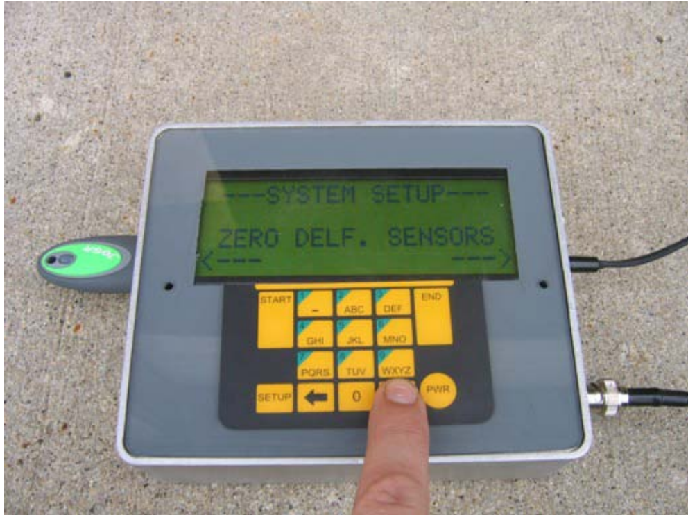
Figure 5.14. System Setup Screen 1 for Prototype Test Roller System (Zero Sensors).
