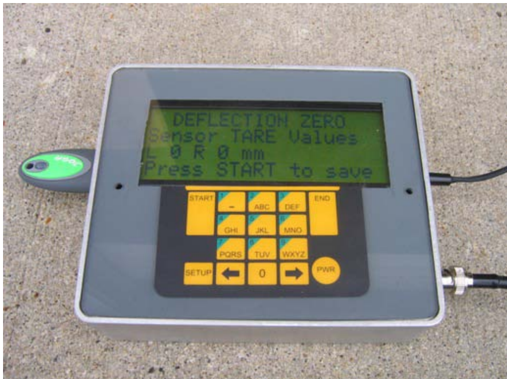
Figure 5.21. Zero Sensors Screen 3 for Prototype Test Roller System (Sensor Tare Values).
