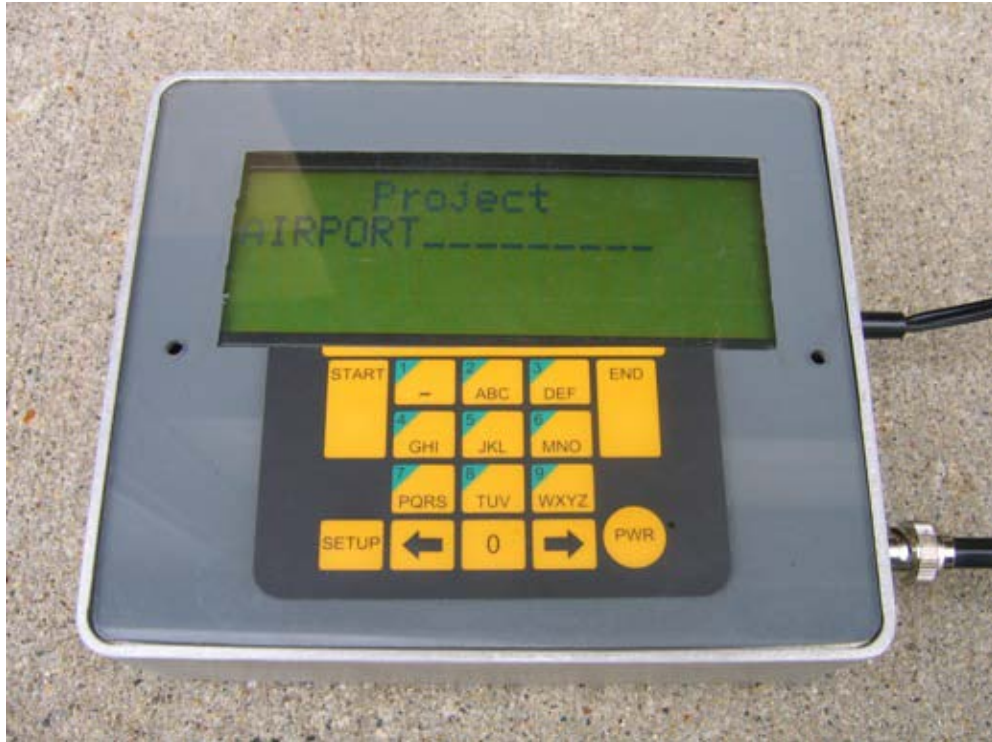
Figure 5.6. Input Screen 5 for Prototype Test Roller System (Project ID).
