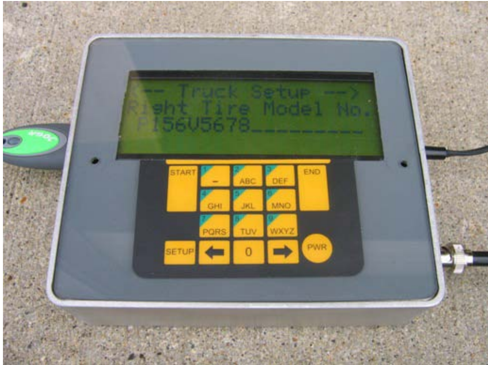
Figure 5.30. Truck Setup Screen 9 for Prototype Test Roller System (Right Tire Model No.).
