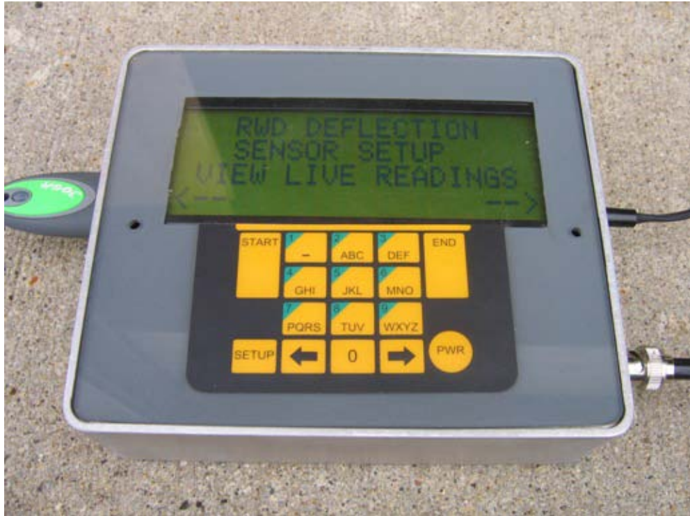
Figure 5.32. Sensor Setup Screen 1 for Prototype Test Roller System (View Live Readings).
