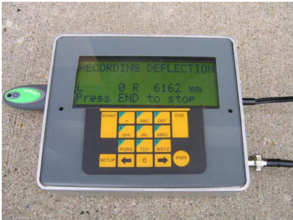
Figure 5.35. Recording Deflection Screen for Prototype Test Roller System.
