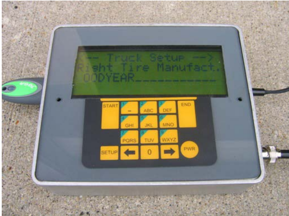
Figure 5.28. Truck Setup Screen 7 for Prototype Test Roller System (Right Tire Manufacturer).
