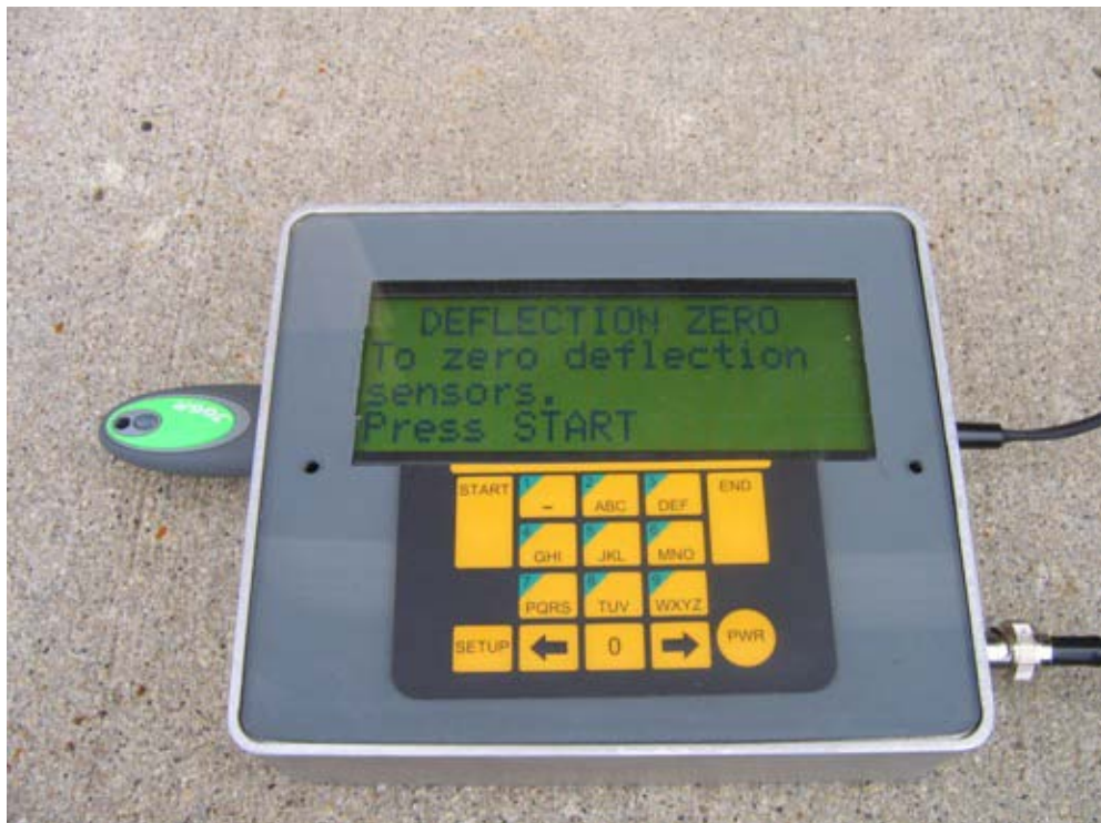
Figure 5.19. Zero Sensors Screen 1 for Prototype Test Roller System (To Zero, Press Start).
