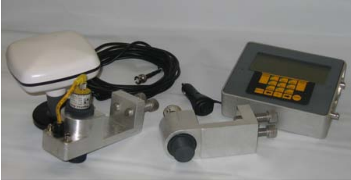
Figure 5.1. Hardware Components of the Prototype Test Roller System.
