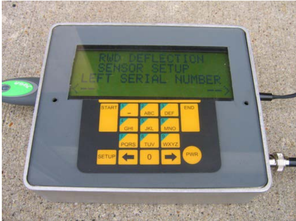
Figure 5.34. Sensor Setup Screen 3 for Prototype Test Roller System (Sensor Serial Number).
