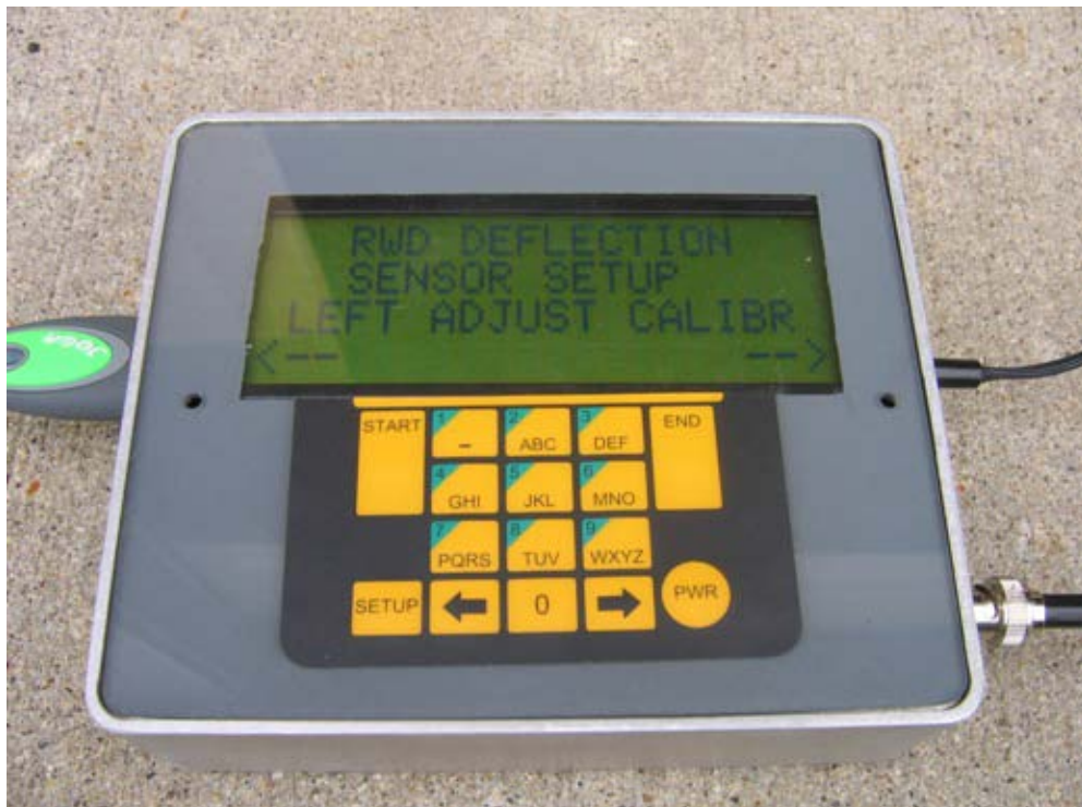
Figure 5.33. Sensor Setup Screen 2 for Prototype Test Roller System (Adjust Calibration).
