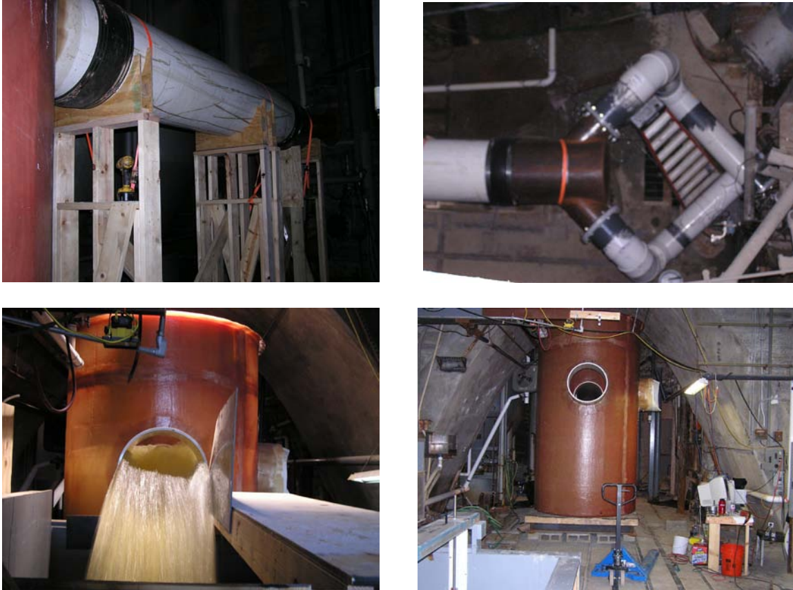
Figure A.4. 6-ft Sump Setup
