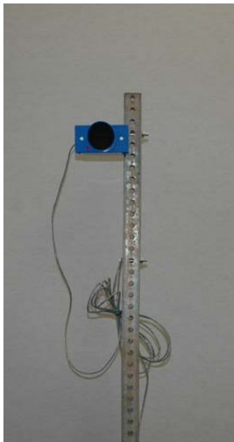
Figure 25: SonaSwitch ultrasonic test circuit.
