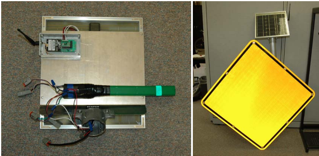
Figure 40: Modified Tapco circuitry (left) and complete blinker sign.
