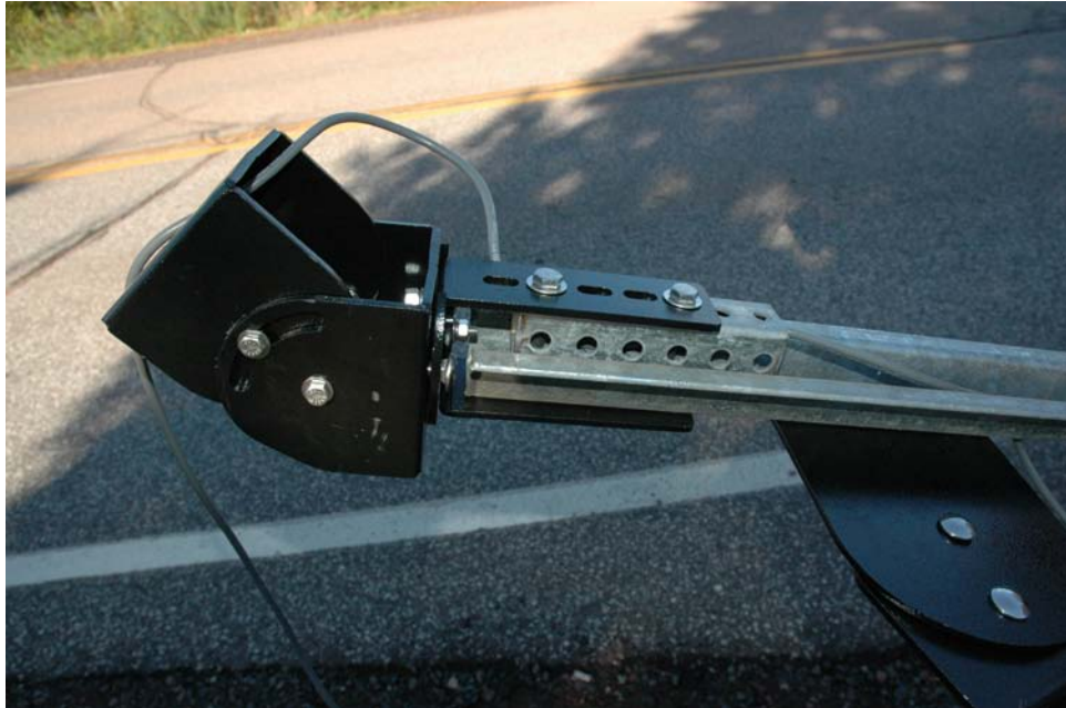
Figure 42: Mounted solar panel and radar sensor brackets.
