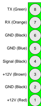
Figure 35: Radar detector 8-pin header.
