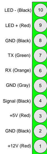
Figure 33: PIR detector 10-pin header.
