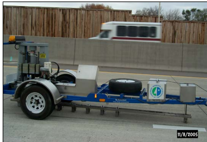
Figure 2 FWD Testing Device
