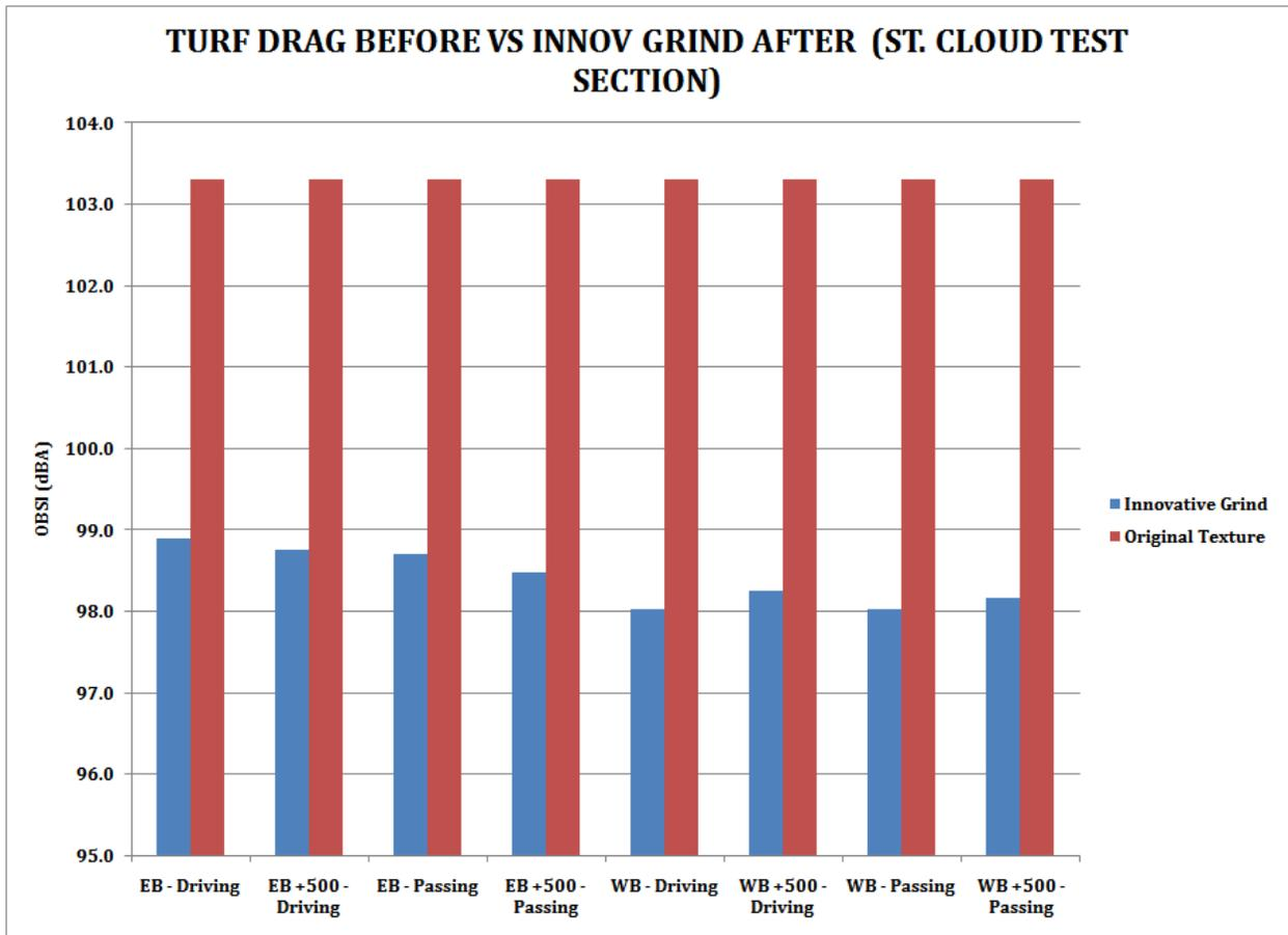
Figure D.33. Innovative grind Versus Original Texture(Before & After Analysis)
