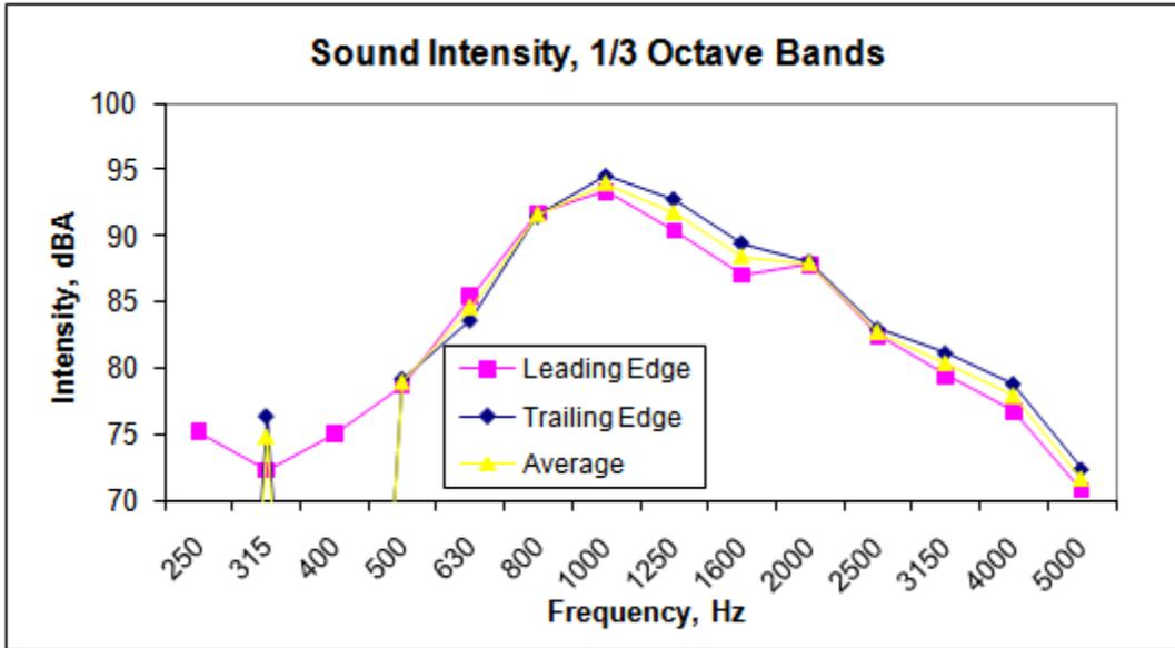
Figure D.38. St. Cloud Test Section EB +500 Innovative Grind Driving Lane Trial 3
