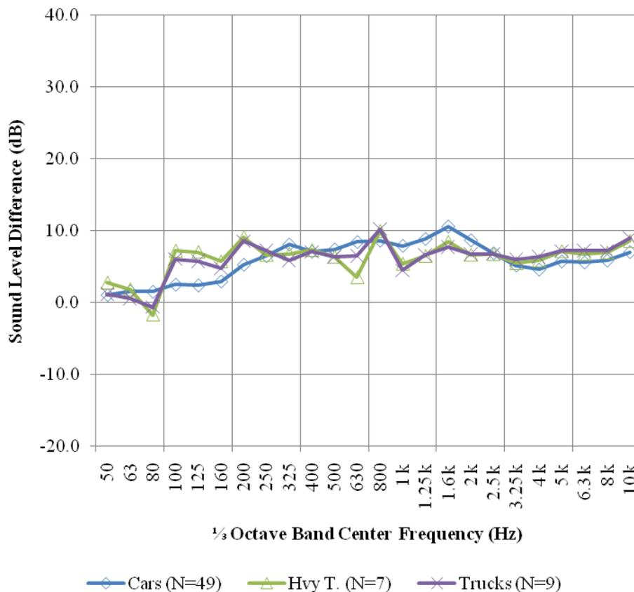
**Figure 7.9.  $L_{veh}$  spectrum (at ref. speed) difference of cell 7 from cell 97 at 25 ft**
