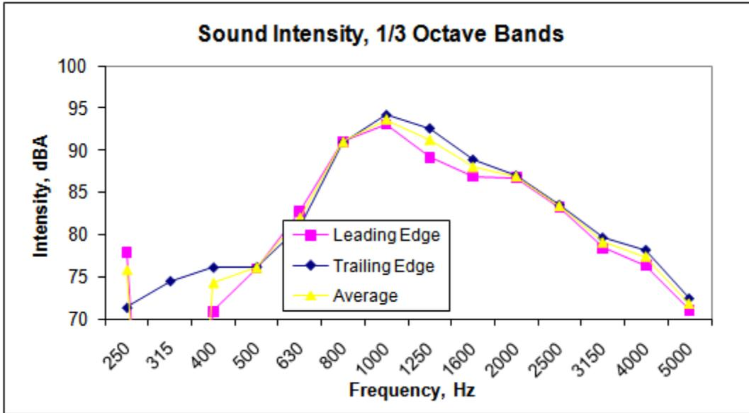
Figure D.62. St. Cloud Test Section WB +500 Innovative Grind Driving Lane Trial 3
