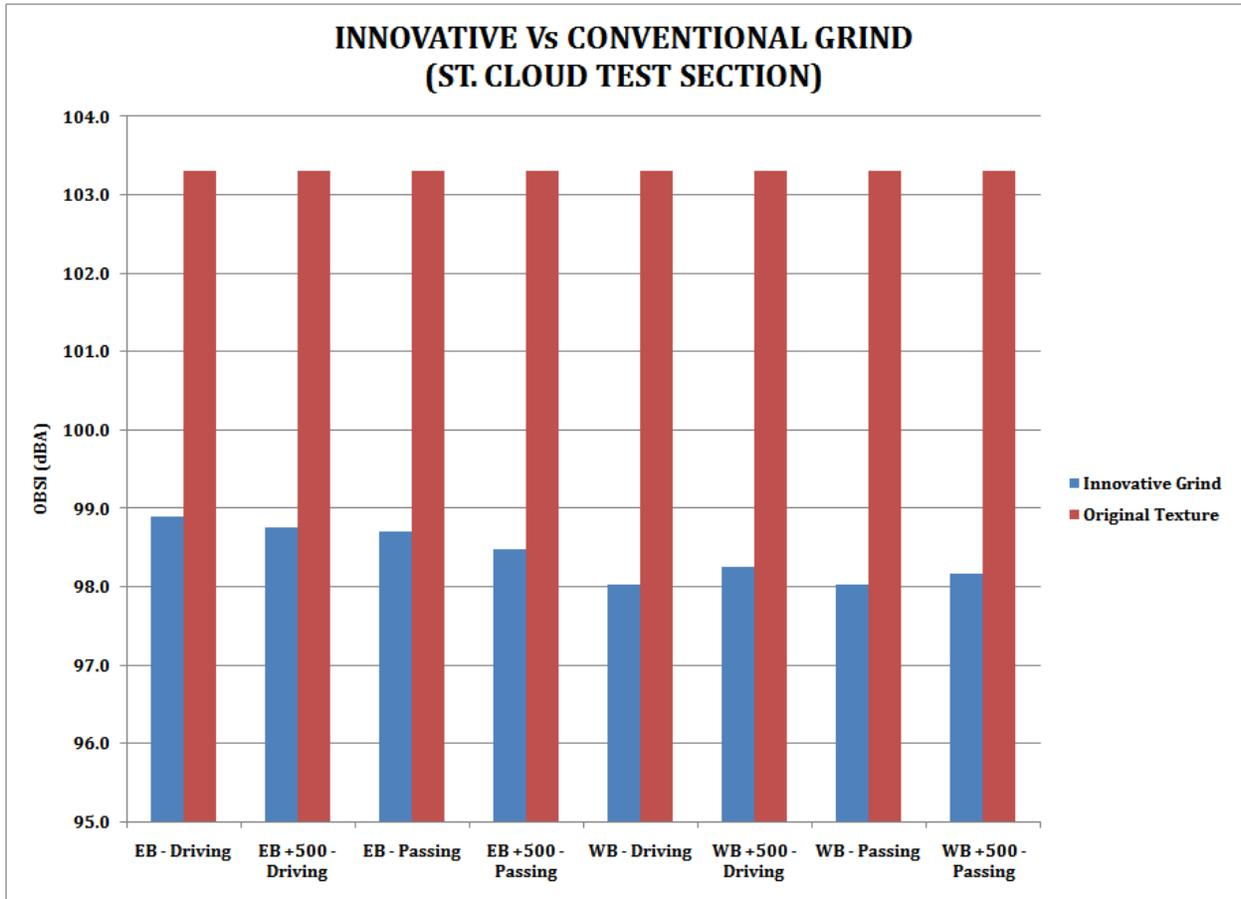
**Figure D.32. Innovative grind Versus Original Texture(Before & After Analysis)**
