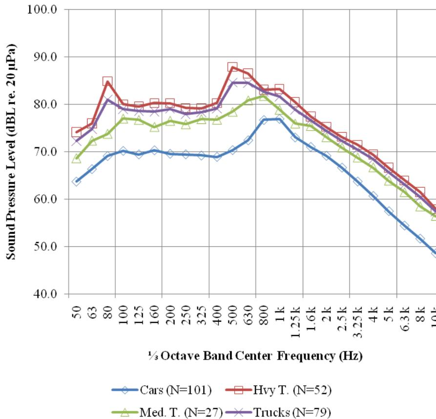
**Figure 7.6.  $L_{veh}$  spectrum (at ref. speed) for subject pavement (innovative grind) at 25 ft**
