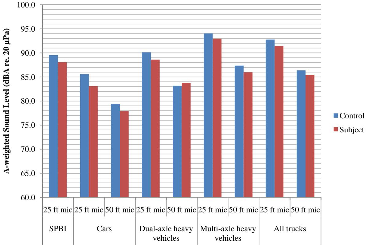
**Figure 8.3. Summary of vehicle sound levels for the control and subject pavements**
