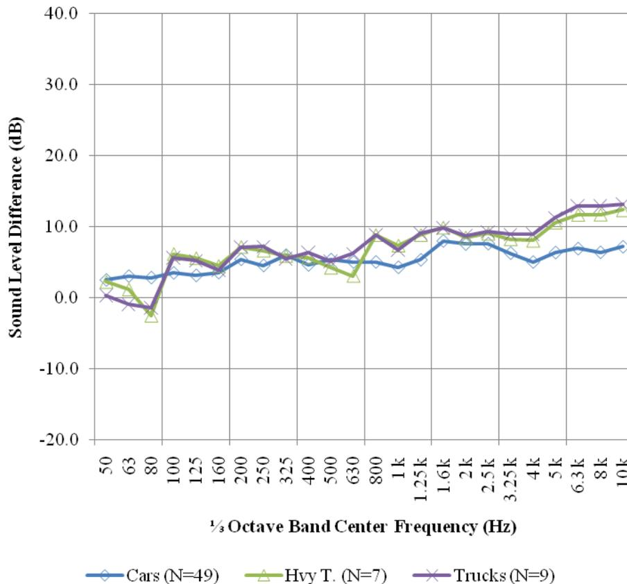
**Figure 7.10.  $L_{veh}$  spectrum (at ref. speed) difference of cell 8 from cell 97 at 25 ft**
