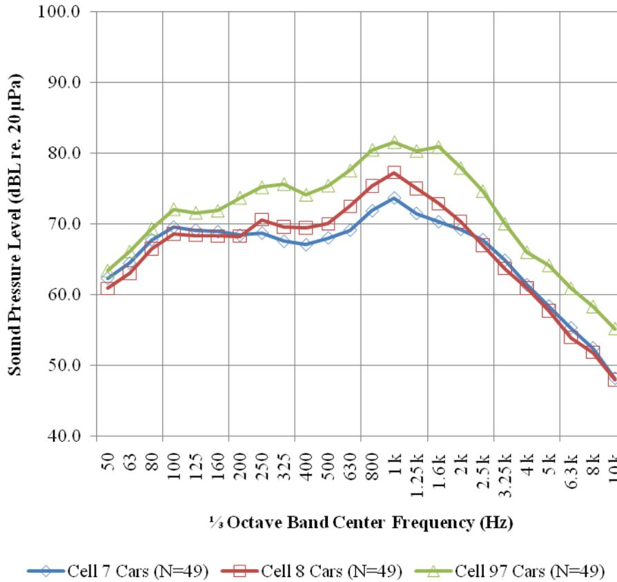
**Figure 8.1. Vehicle category 1 (cars) comparison of MnROAD test cells**
