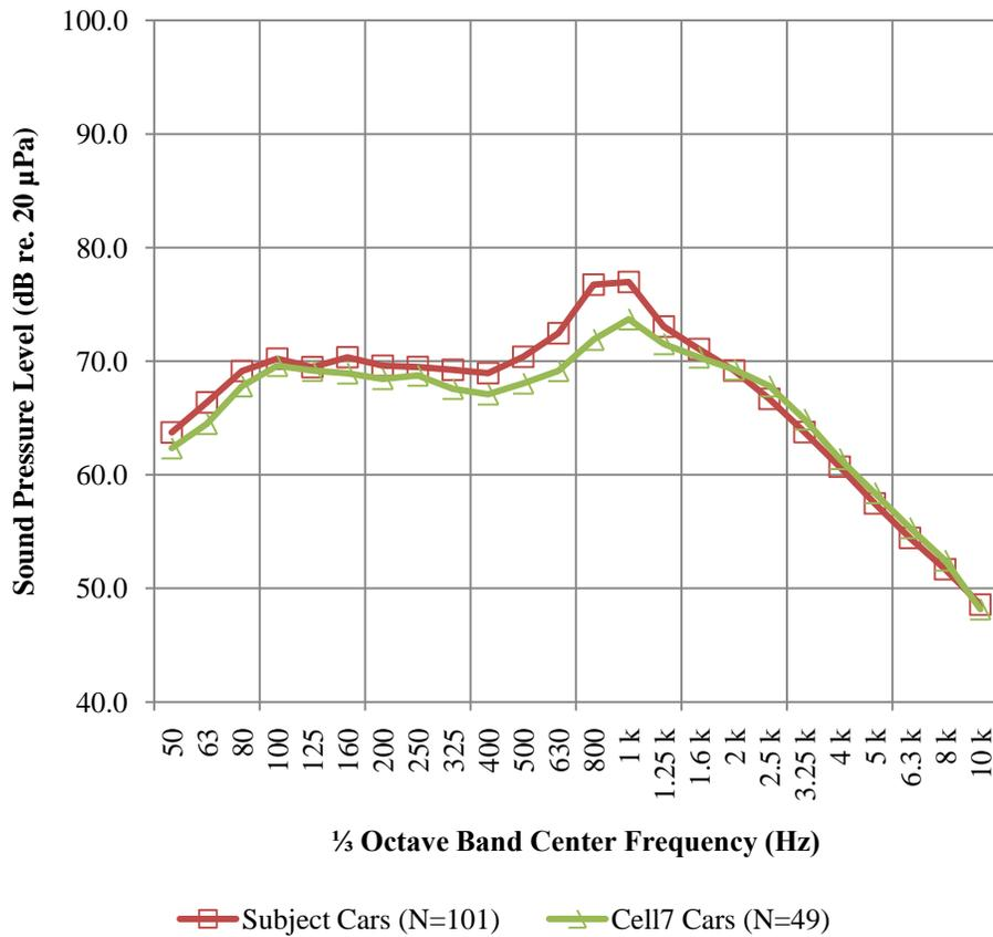
**Figure 8.6. Vehicle category 1 (cars) MnROAD test cell 8 versus subject pavement on I-94**
