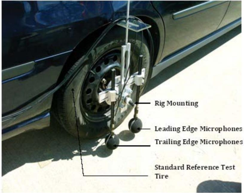
**Figure D.1: OBSI Assembly showing SRTT, Mounting Rig, Microphones and Cables**
