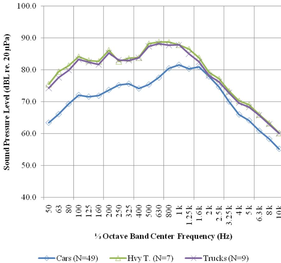
**Figure 7.3.  $L_{veh}$  spectrum (at ref. speed) pavement cell 97 (transverse tine) at 25 ft**
