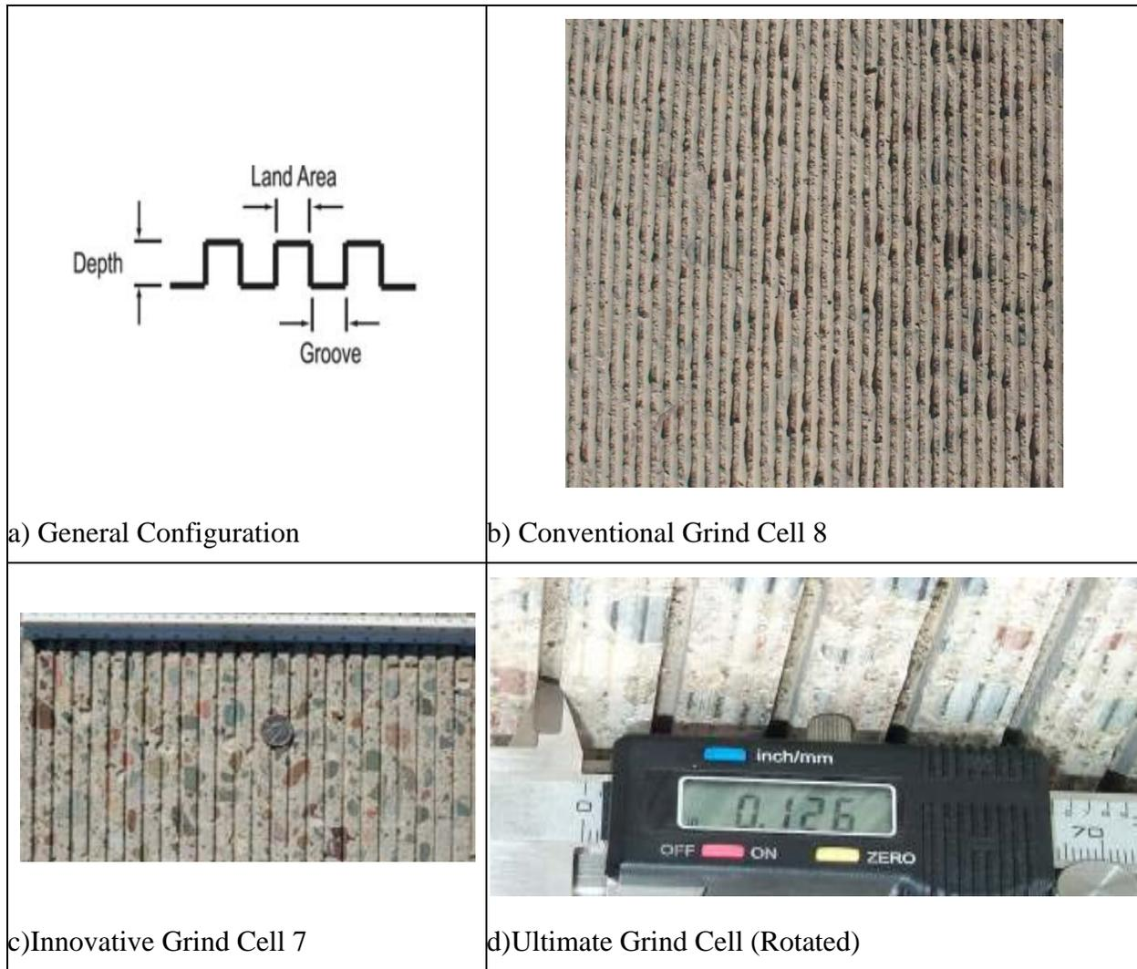
Figure A.1. General Diamond Grinding Configuration Nomenclature and three Grinding Configurations
