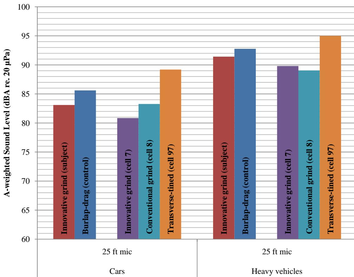
**Figure ES.1. Overall comparison of SPB measurements**
