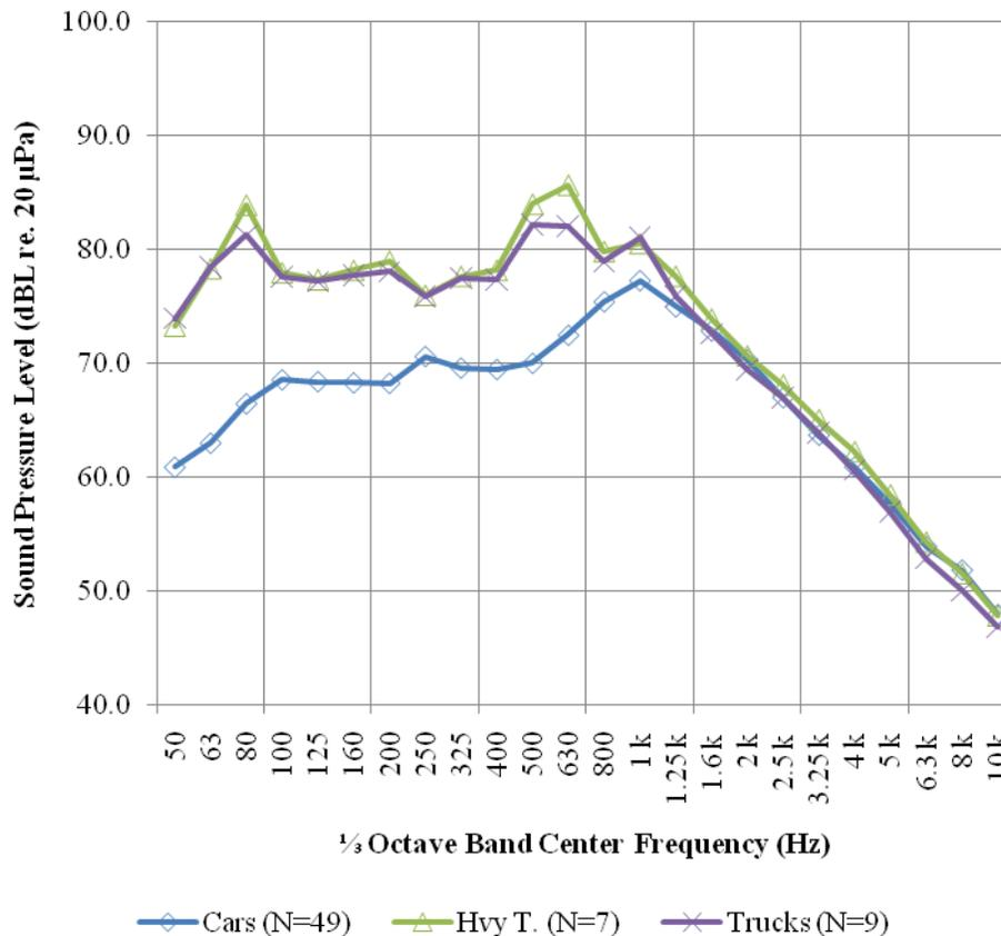
**Figure 7.2.  $L_{veh}$  spectrum (at ref. speed) pavement cell 8 (conventional grind) at 25 ft**
