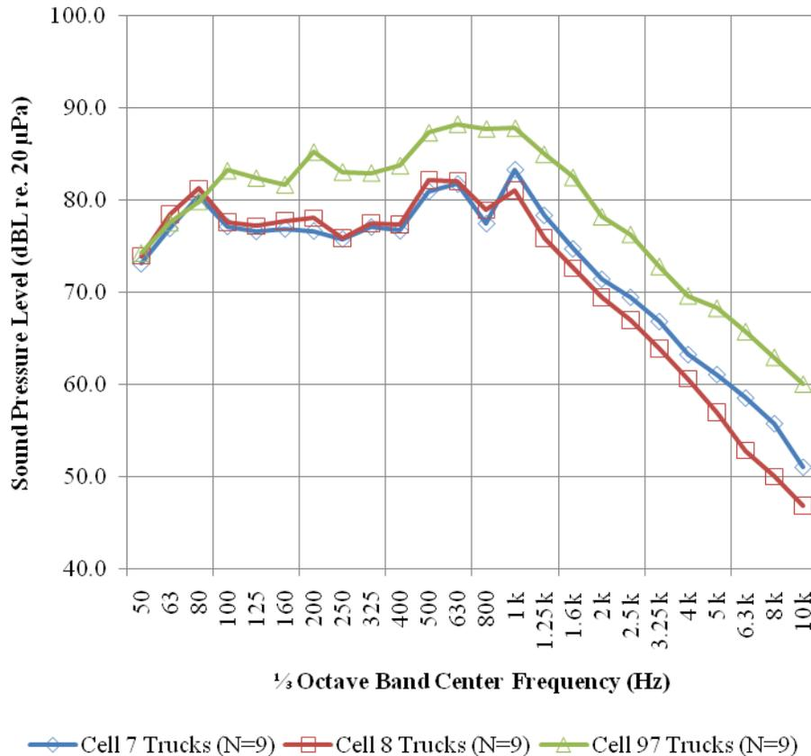
**Figure 8.2. Vehicle category 2 (all trucks) comparison of MnROAD test cells**
