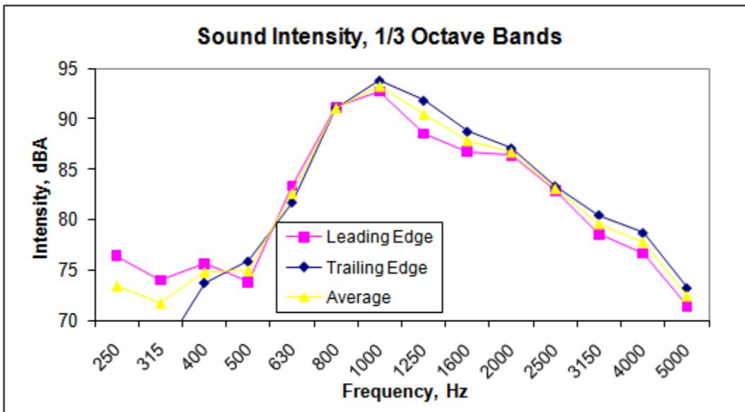
Figure D.57. St. Cloud Test Section WB Innovative Grind Driving Lane Trial 1
