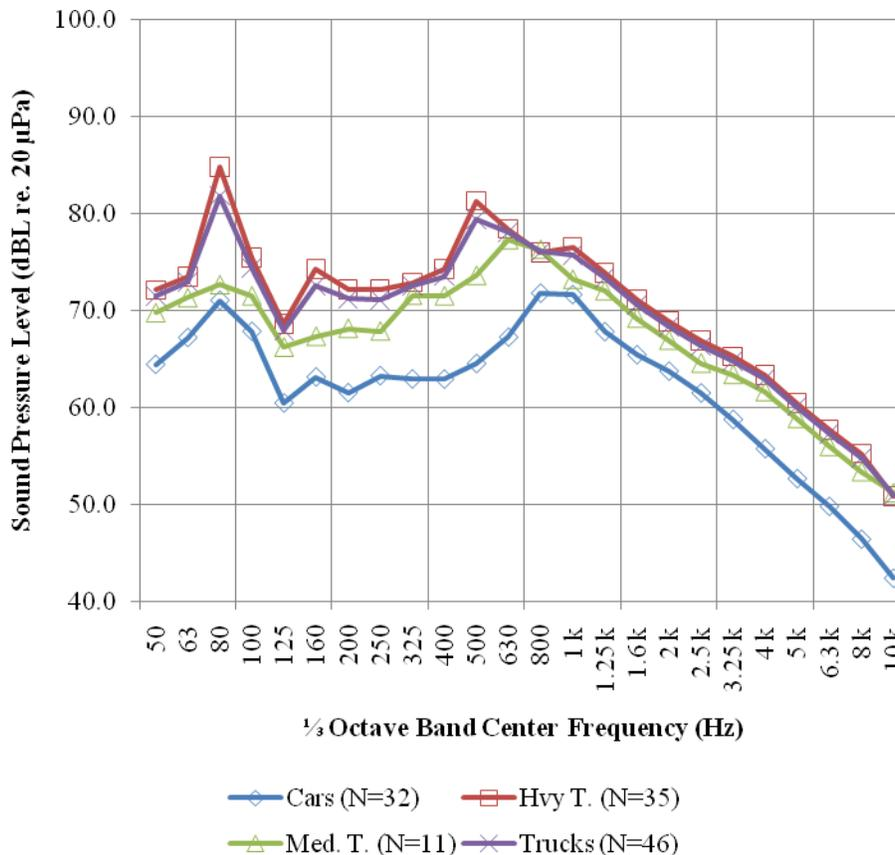
**Figure 7.7.  $L_{veh}$  spectrum (at ref. speed) for subject pavement (innovative grind) at 50 ft**
