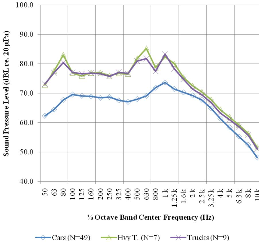
**Figure 7.1.  $L_{veh}$  spectrum (at ref. speed) pavement cell 7 (innovative grind) at 25 ft**
