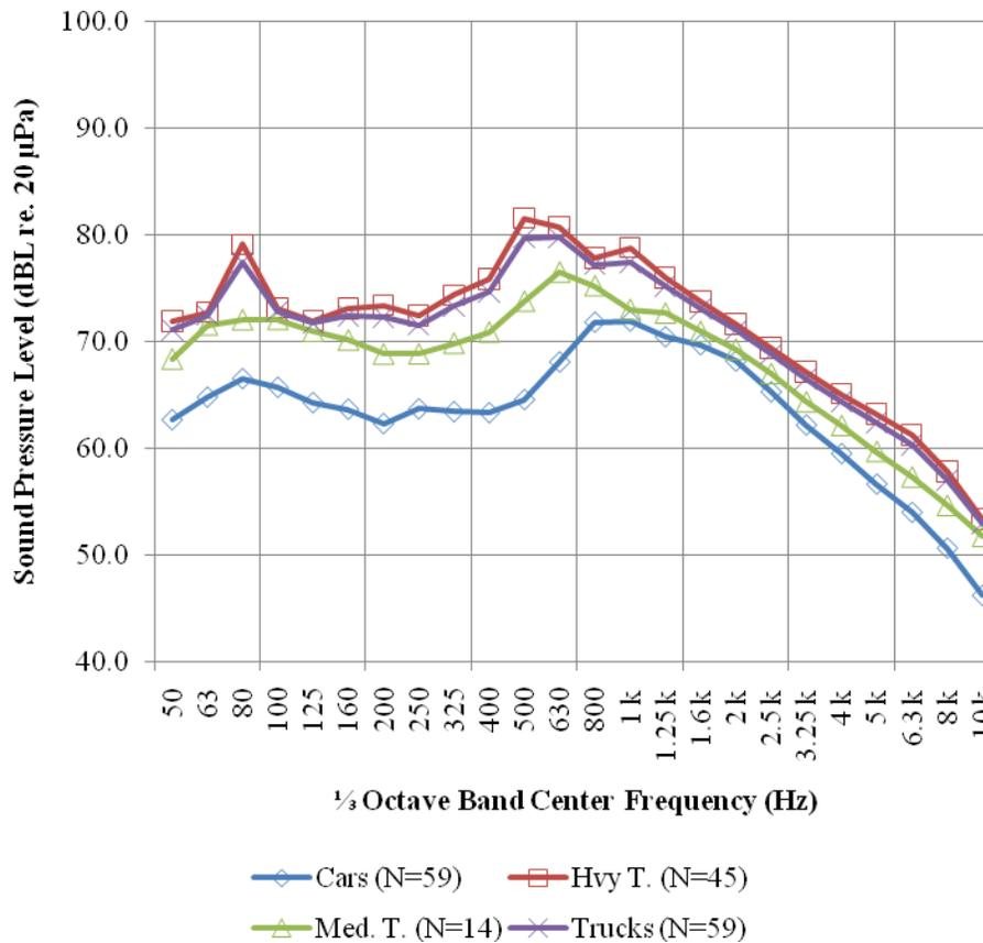
**Figure 7.5.  $L_{veh}$  spectrum (at ref. speed) for control pavement (burlap drag) at 50 ft**
