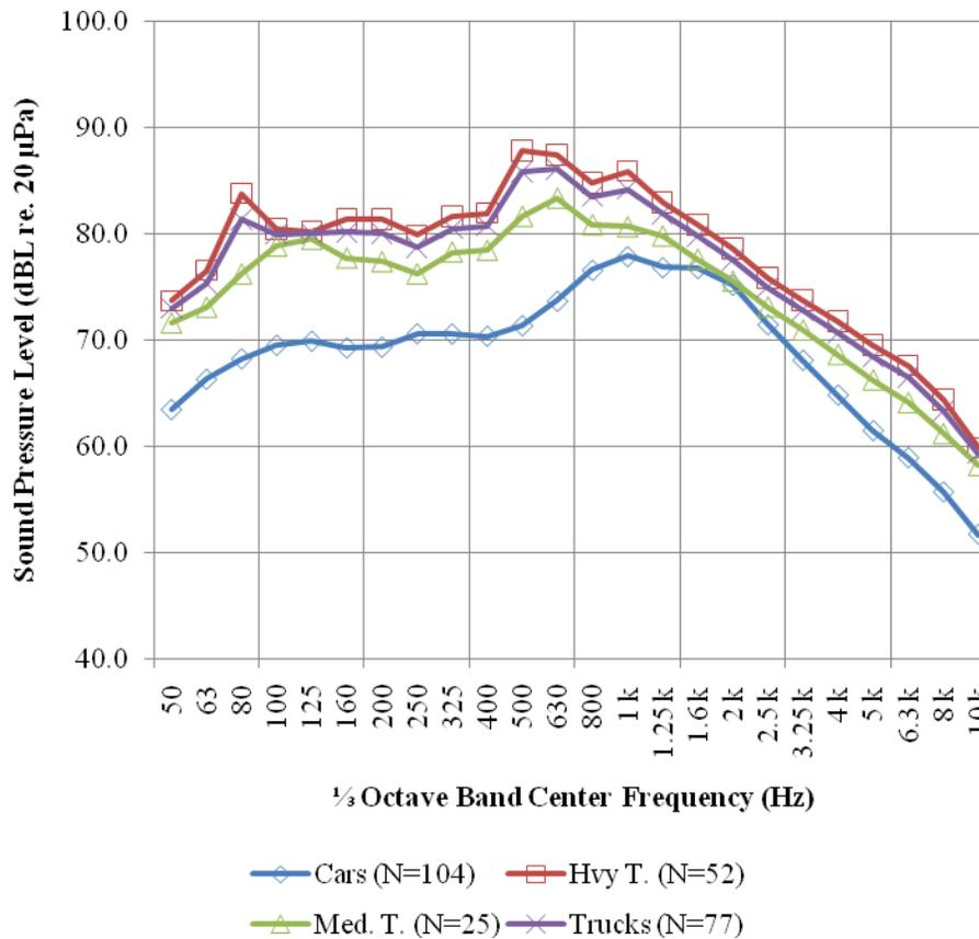
**Figure 7.4.  $L_{veh}$  spectrum (at ref. speed) for control pavement (burlap drag) at 25 ft**
