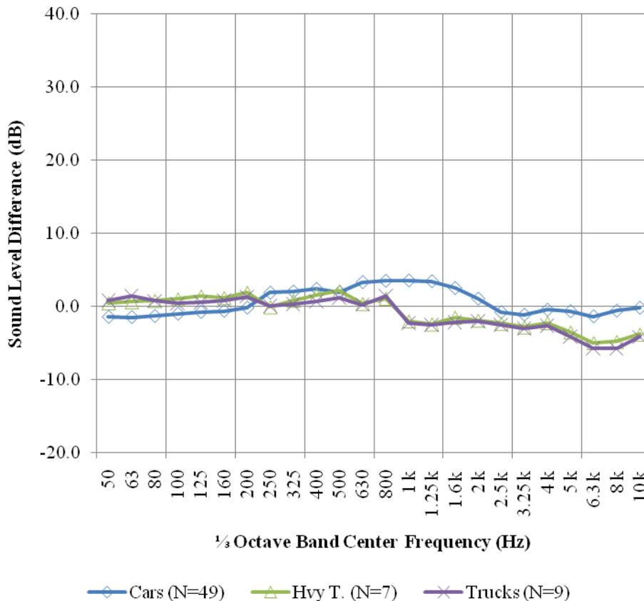
**Figure 7.8.  $L_{veh}$  spectrum (at ref. speed) difference of cell 7 from cell 8 at 25 ft**
