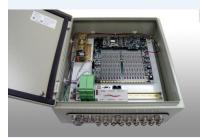
Waterproof housings allow for on-site installation of electronics necessary to power the sensors and acquire data.
