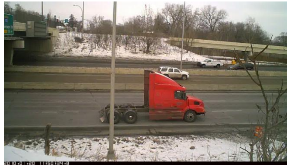
Class 6 truck classified as PV by the GTT Canoga Microloops.
