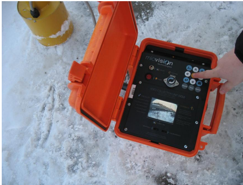
Figure 35. Miovision VCU with Video Display
