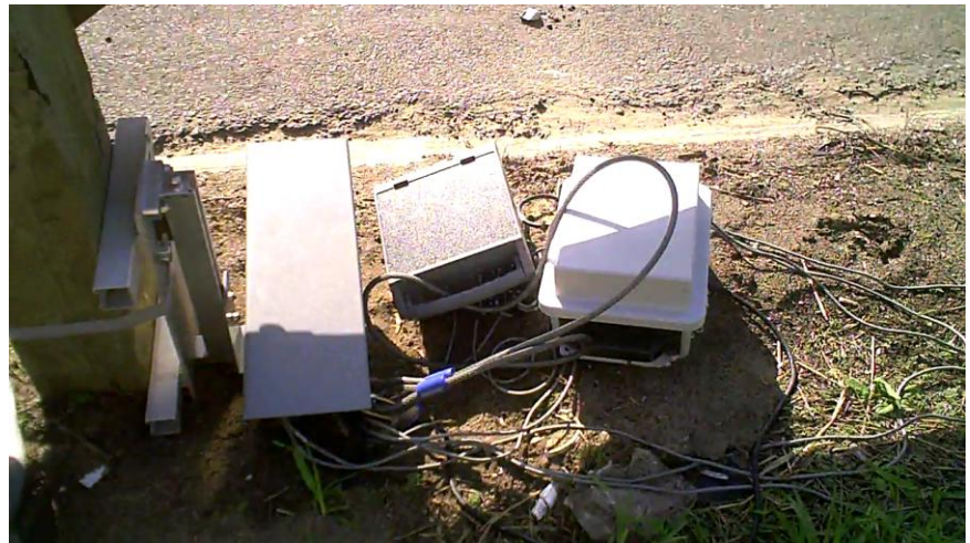
AxleLight, PEEK ADR 1000 and battery module.
