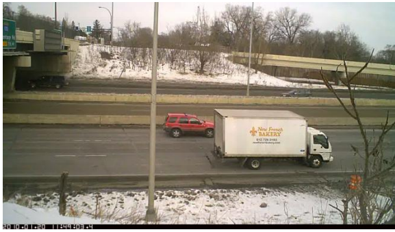
Small Class 5 truck classified as PV by the GTT Canoga Microloops.
