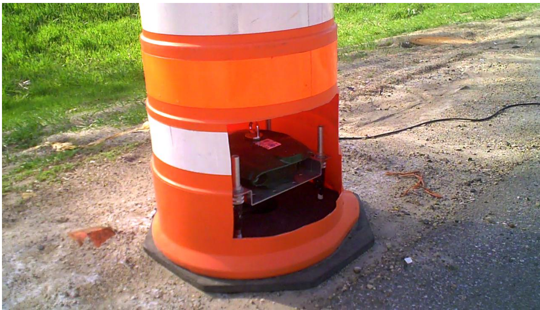
Figure 24. Traffic Barrel with Cutout for TIRTL Sensor.
