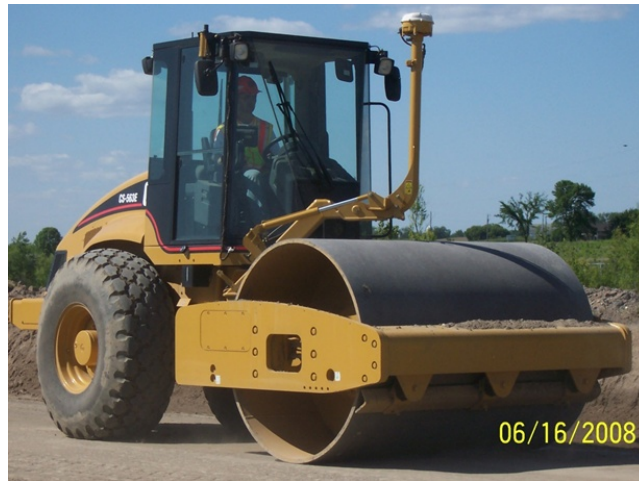
Figure 2—Caterpillar Roller Used for 2008 MnRoad IC Measurements
