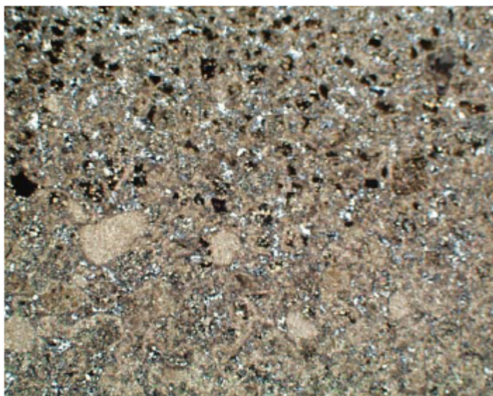
Fig. 10: Photomicrograph (crossed polars; 10.5mm X 8mm) of aggregate displaying a transition (top to bottom) from Type I mineralogy to Type II mineralogy.
