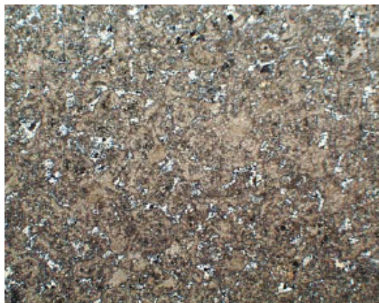
Fig. 4: Photomicrograph (crossed polars; 10.5mm X 8mm) of a minnesotaite-rich aggregate. Minnesotaite-rich areas are tan in color.
