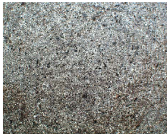
Fig. 14: Photomicrograph (crossed polars; 10.5mm X 8mm) of cherty siderite. Though grains are indistinguishable, the mass has a greyish hue in thin section from the high concentration of chert.
