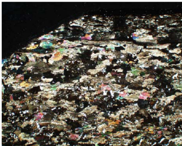
Fig. 15: Photomicrograph (crossed polars; 10.5mm X 8mm) of a meta-siderite-rich aggregate. Tan and multi-colored zones are composed of coarse-grained siderite. Black-colored zones are also composed of coarse-grained siderite but appears extinct.
