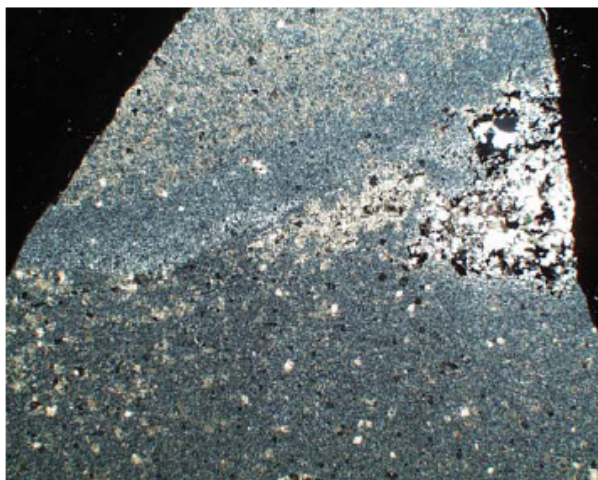
Fig.11: Photomicrograph (crossed polars; 10.5mm X 8mm) of a chert aggregate. Minnesotaites are concentrated in the upper third of the slide, euhedral siderite/dolomite crystals are visible in the lower half of the slide, and coarse carbonate is present in a wedge on the right fringe of the particle.
