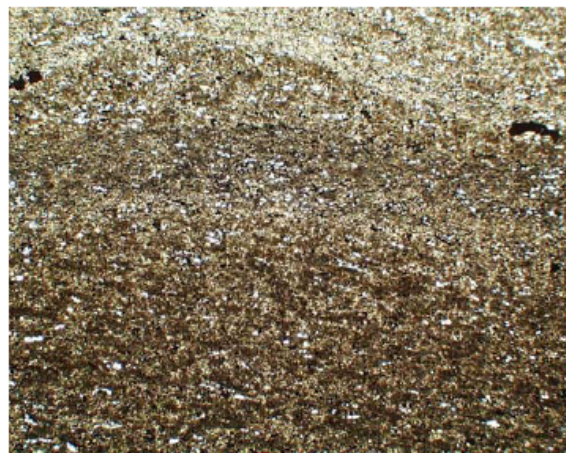
Fig. 13: Photomicrograph (crossed polars; 10.5mm X 8mm) of siderite-rich aggregate. Brown areas are composed mainly of siderite and clear to white zones are quartz/chert.
