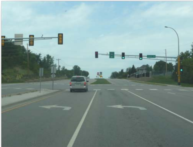
Example Dual Left Turn Lane Design
